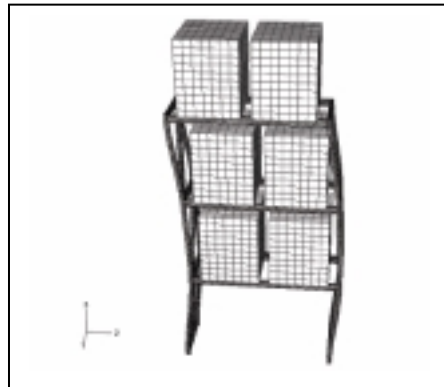
Figure 6 Third Mode Shape of Rack
