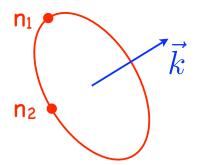
The polarization directions that have a max and min index of refraction form the major and minor axes of an ellipse defining  $n(\theta)$  the index for wave with the electric displacement vector at an angle of  $\theta$  in the transverse plane.
