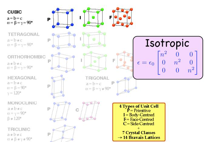
The geometry of a crystal determines the form of the dielectric tensor
