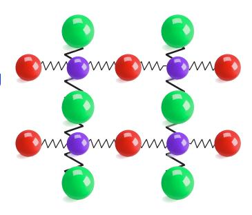
The wells of the electrostatic potential that the charges sit in are not symmetric and therefore the material response (material polarization) is not necessarily in the direction of the driving field.
