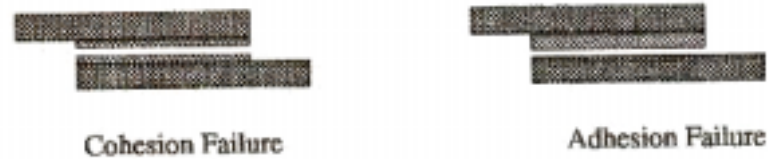
Figure 1: An illustration of adhesive and cohesive failures
