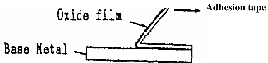
Figure 15. Tape peel test [7]
