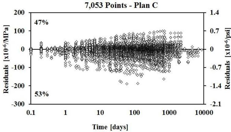
Figure 17-NU-ITI creep compliance residuals for GL 2000 model for 0-10,000 days
