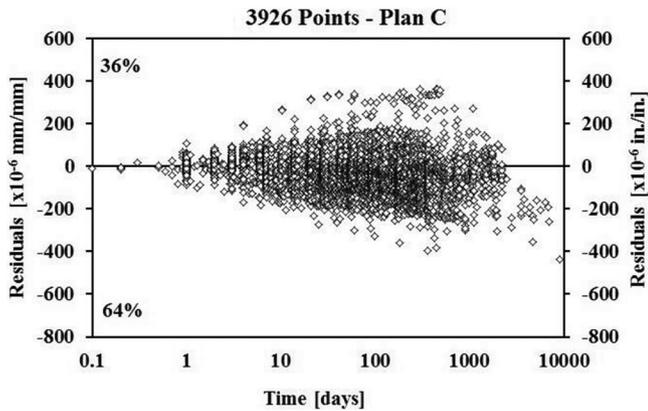
Fig. 4—RILEM shrinkage strain residuals for B3 model for 0 to 10,000 days.
