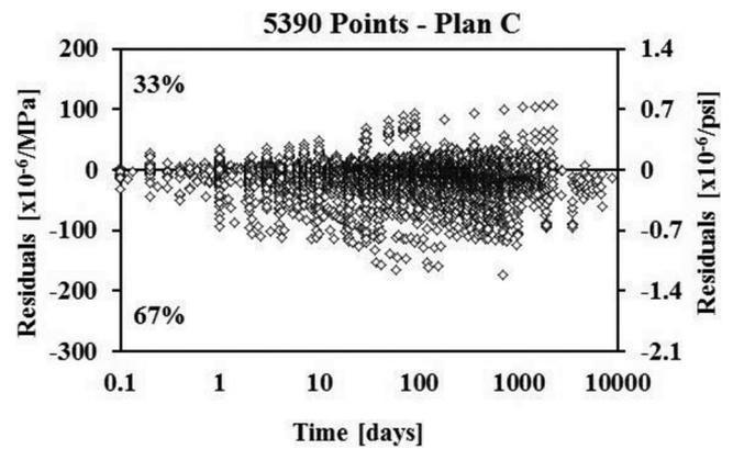
Fig. 7—NU-ITI creep compliance residuals for ACI 209R-92 model for 0 to 10,000 days.
