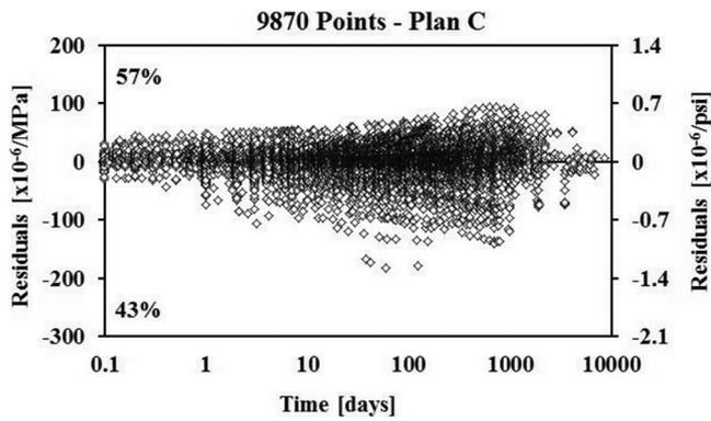
Fig. 10—RILEM creep compliance residuals for B3 model for 0 to 10,000 days.
