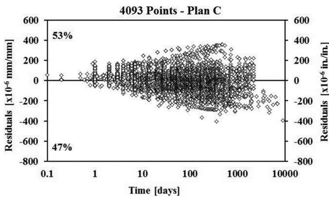
Fig. 5—NU-ITI shrinkage strain residuals for CEB MC 90-99/fib MC 2010 model for 0 to 10,000 days.
