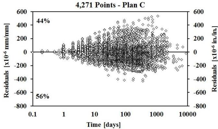
Figure 13-NU-ITI shrinkage strain residuals for GL 2000 model for 0-10,000 days
