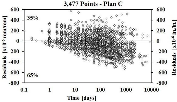
Figure 16-RILEM shrinkage strain residuals for AASHTO 2012 model for 0-10,000 days
