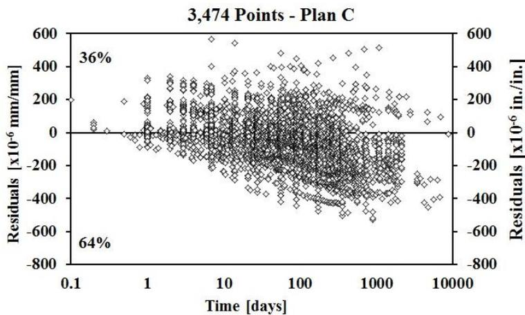
Figure 15-NU-ITI shrinkage strain residuals for AASHTO 2012 model for 0-10,000 days
