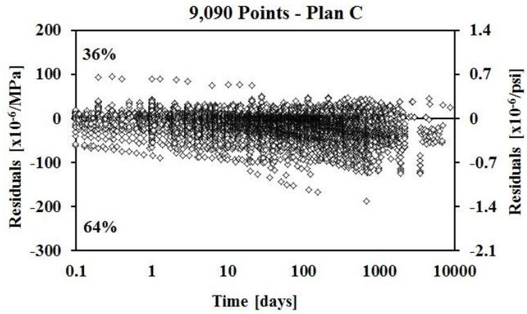
Figure 22-RILEM creep compliance residuals for AASHTO 2012 model for 0-10,000 days
