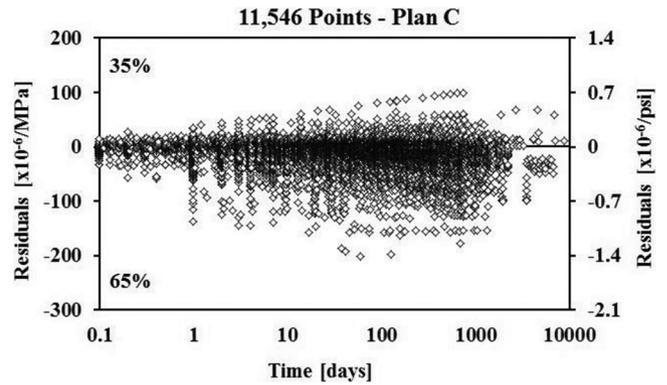
Fig. 12—RILEM creep compliance residuals for fib MC 2010 model for 0 to 10,000 days.
