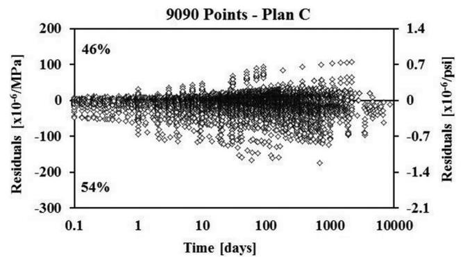
Fig. 8—RILEM creep compliance residuals for ACI 209R-92 model for 0 to 10,000 days.
