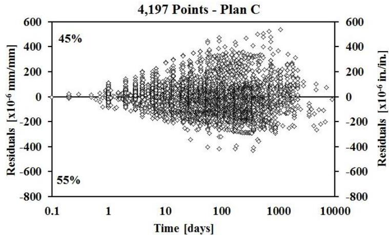
Figure 14-RILEM shrinkage strain residuals for GL 2000 model for 0-10,000 days
