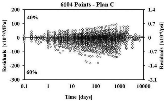
Fig. 9—NU-ITI creep compliance residuals for B3 model for 0 to 10,000 days.
