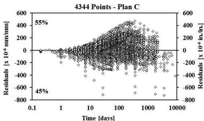
Fig. 1—NU-ITI shrinkage strain residuals for ACI 209R-92 model for 0 to 10,000 days.
