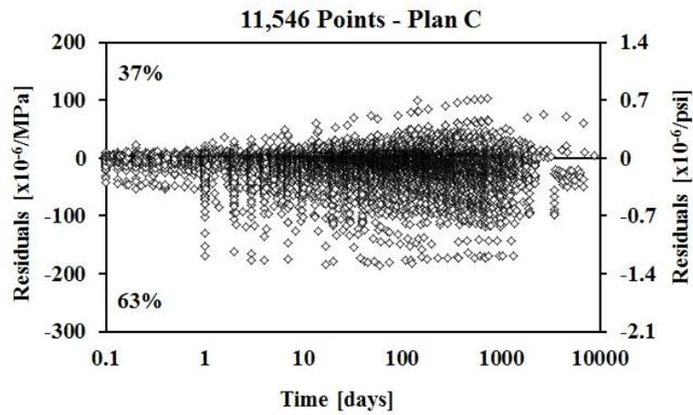
Figure 20-RILEM creep compliance residuals for CEB MC 90-99 model for 0-10,000 days
