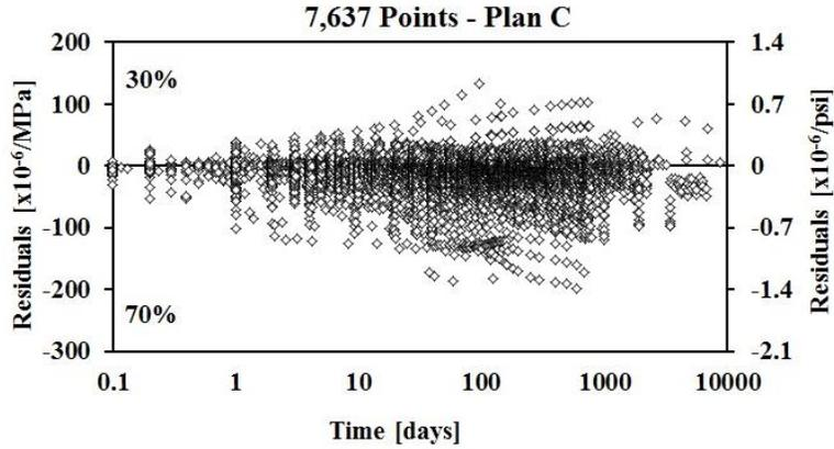
Figure 19-NU-ITI creep compliance residuals for CEB MC 90-99 model for 0-10,000 days
