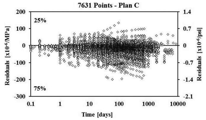
Fig. 11—NU-ITI creep compliance residuals for fib MC 2010 model for 0 to 10,000 days.
