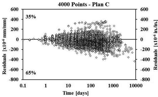
Fig. 3—NU-ITI shrinkage strain residuals for B3 model for 0 to 10,000 days.
