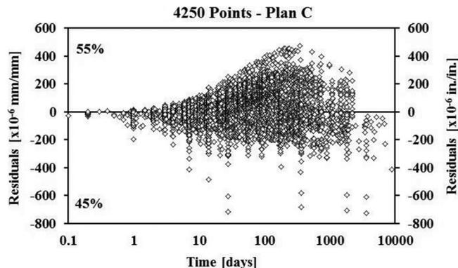
Fig. 2—RILEM shrinkage strain residuals for ACI 209R-92 model for 0 to 10,000 days.
