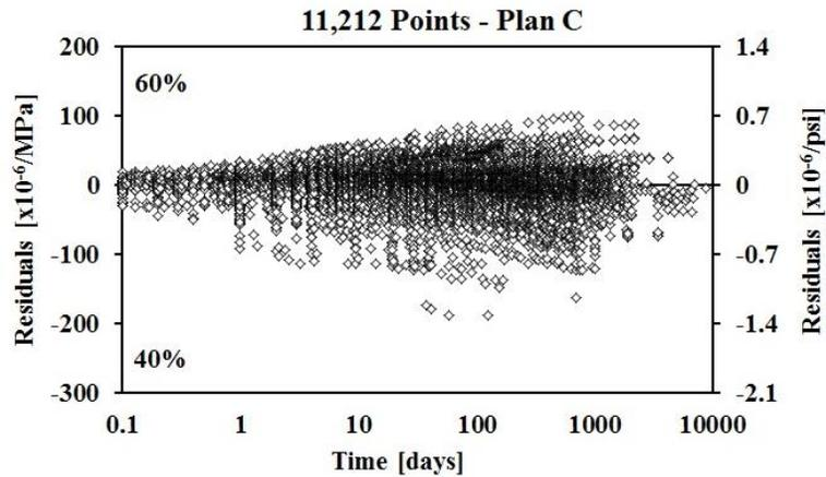
Figure 18-RILEM creep compliance residuals for GL 2000 model for 0-10,000 days
