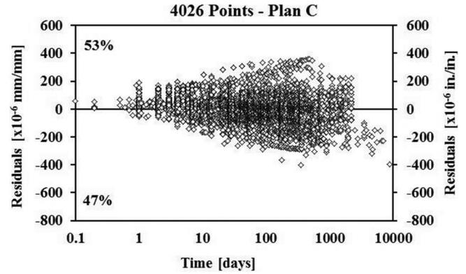
Fig. 6—RILEM shrinkage strain residuals for CEB MC 90-99/fib MC 2010 model for 0 to 10,000 days.
