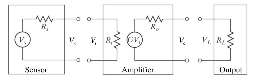
□ Connecting an amplifier to a sensor can change what would otherwise have been the original signal  $V_s$ , because a new circuit loop is made. Likewise a problem at the output. Circuit analysis shows:
