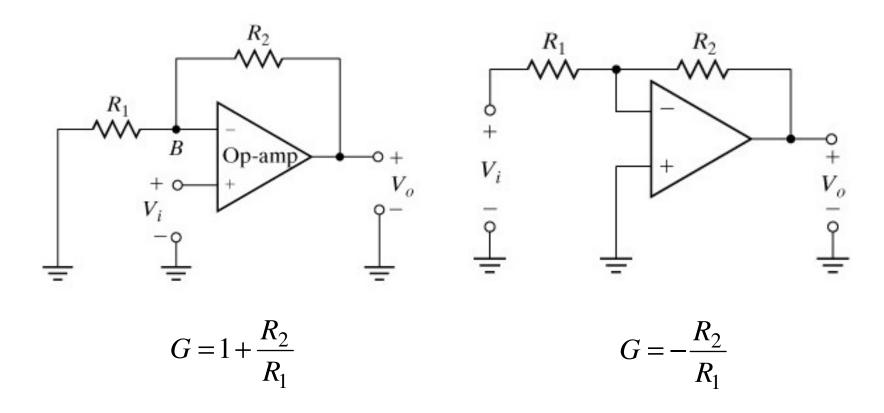
□ Commercial op-amps readily can have gain >  $10^5$ , CMRR near 100 dB, input impedance >  $10^5 \Omega$ , and output impedance <  $100 \Omega$ . Why are these good?
