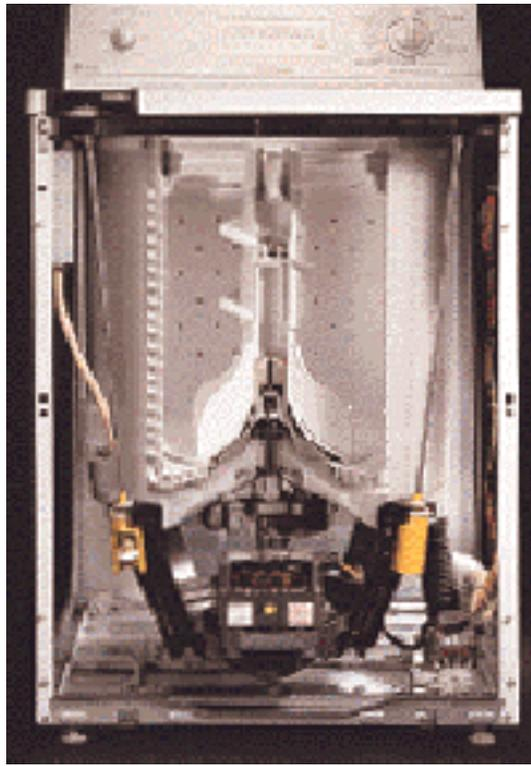
*principles, General Electric's Profile Super 32 clothes washer features a sensor-based feedback control that maintains correct water temperature no matter the load size*
