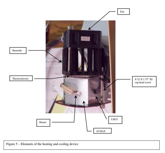
In this code, the operation of the system was to heat up to 60 °C then turn the heater off, turn the cooling system on, cool to 30 °C then turn the cooling system off then loop around again. This approach did not work for three reasons: 1) the SDAS board I had built had malfunctioned and 2) the functions located in sdasapi.h would not load on my compiler 3) the A2D conversion may have had to have been in the form of a voltage not a digital value. The compiler used was Borland Turbo C++ 4.5.
