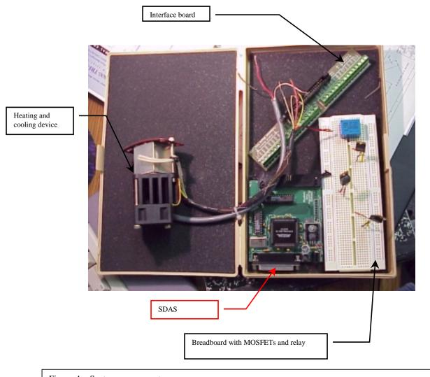
Figure 4 – System components
