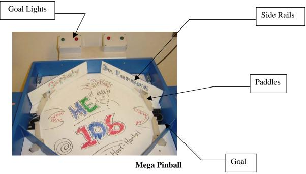
Figure 6. Top view of actual game board with components.
