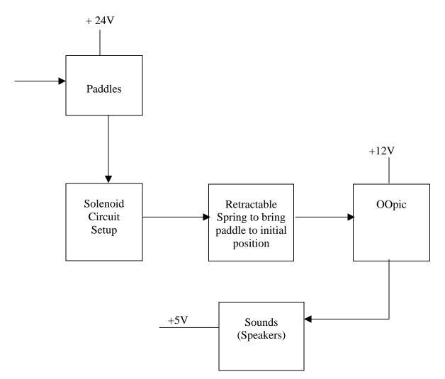
Figure 4. Block diagram of operating solenoids (paddles).
