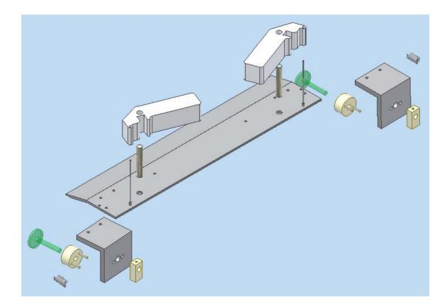
Figure 7. Exploded View of Solenoid Paddle Mechanism
