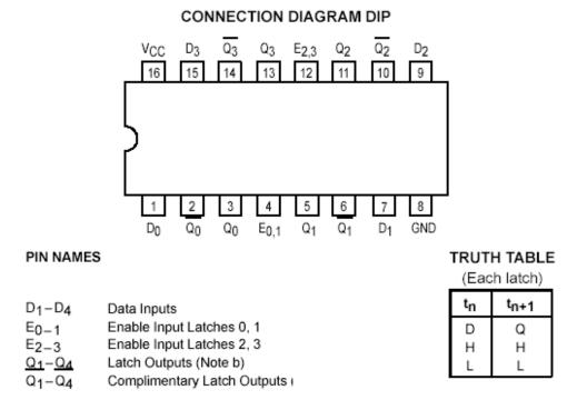
Figure 12. IC chip 74LS375, 4Bit D-latch, temporary storage for binary input/output
