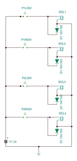
Figure 9. Connection Circuitry for the paddle electric solenoid.
