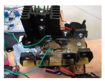
Figure 3: Actual H-Bridge Circuit
