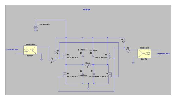
Figure 2: H-Bridge Schematic
