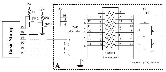
Figure 3 Switch-controlled display circuit.
