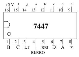
**Figure 2** 7447 BCD-to-7-segment decoder driver chip. This chip takes a 4-bit binary number applied to DCBA, where A is the least significant bit (LSB), and grounds the appropriate pin 9-15, so that when these pins are connected to a 7-segment LED display through current limiting resistor, the corresponding decimal number will appear on the display. The 7447 is used to drive common anode (CA) displays.
