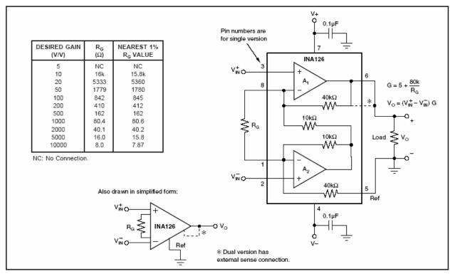
Figure 5 INA126 pinout and guide to configuring its gain. One resistor,  $R_G$ , is all that is needed to set the gain of the amplifier, which can range from 5 to 10,000. The internal connections of the pins are shown. Note that the actual physical location of the pins does not correspond to the location shown in the drawing. The ordering of pins 1-8 around the edges of the INA126 is like that for the chips shown in Figure 1.
