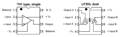
**Figure 1 Examples of single and dual op-amp IC packages.** The '741 was one of the earlier, but still very common, general purpose IC op-amps. Both the '741 and LF353 should be powered with symmetrical positive and negative power supplies (see their data sheets for maximum limits). We will use the LF353 dual op-amp in this experiment.
