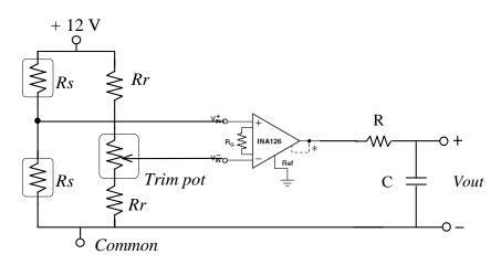
**Figure 6** The electronic scale circuit with low-pass filter. The low-pass filter will attenuate high frequency noise.
