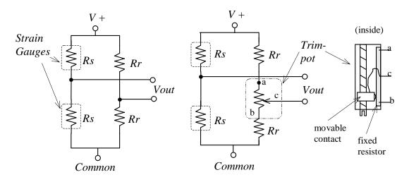
**Figure 4** Wheatstone bridge (left) and Wheatstone bridge with offset adjustment (right). The construction of the trimpot (variable resistor) is also shown.
