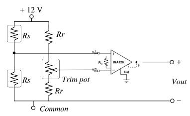
**Figure 6** The electronic scale circuit schematic. The strain gauges are placed in a Wheatstone bridge, and an instrumentation amplifier amplifies the bridge voltage. Although not shown, the supply voltages for the INA126 are  $\pm 12$  V.
