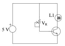
Figure PL-1 Lamp Control Circuit
