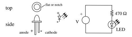
Figure 1 LED circuit
