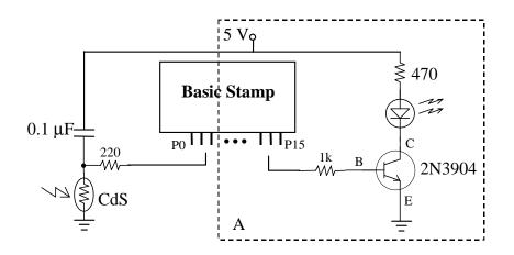
Figure 5 Light-Controlled Switch Using the Basic Stamp
