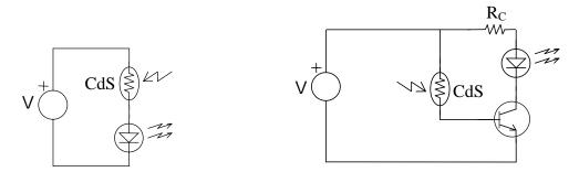
Figure 2 Light-controlled LED Figure 3 Light-controlled using a transistor "switch"
