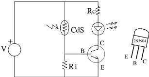
Figure 4 Improved Light-Controlled Switch Using a Transistor
