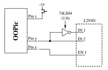
Figure 4. Connections to the OOPic, the 74LS04, and the L293D. Note that the connections for  $V_S$  and +5 are not shown on the L293D, but need to be connected.
