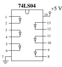
**Figure 2**. 74LS04 connections. The 74LS04 is a logic IC containing six inverters, also called NOT gates. The schematic symbol for a NOT gate is a triangle with an open circle at the end.
