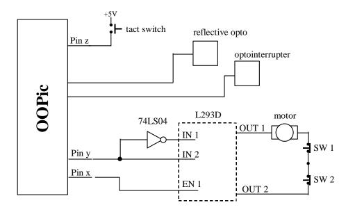
**Figure 5**. Printer Carriage Motion Controller. The carriage is driven between limits set by the two opto-switches continuously after the program detects that the tact switch has closed. The carriage stops when the tact switch is pressed again.
