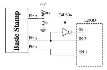
**Figure 4**. Connections to the Basic Stamp, the 74LS04, and the L293D. Note that the connections for  $V_S$  and +5 are not shown on the L293D, but need to be connected.
