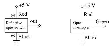
**Figure 1**. Opto-switch connections for photoreflective and photointerrupter switches
