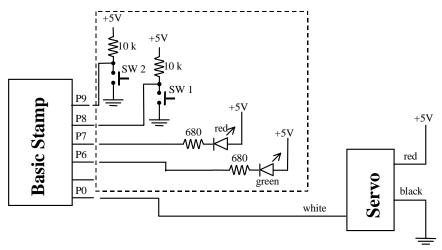
Figure 3 Servo Control Circuit.
