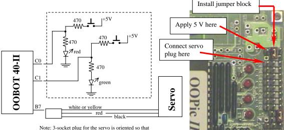
Note: 3-socket plug for the servo is oriented so that black wire is toward the <u>edge</u> of the OOBOT board.
