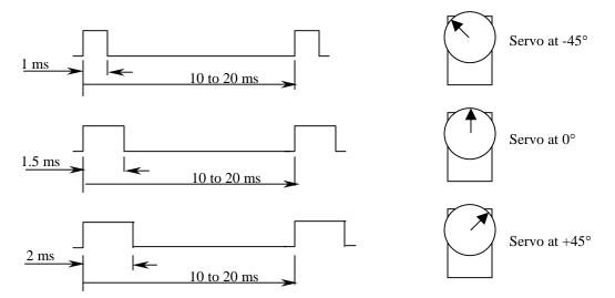
**Figure 2** R/C Servo Operation. The R/C servo needs to see a pulse-width modulated control signal in order to position the output shaft. Pulse-widths vary between approximately 1ms - 2 ms, and have a period of 10 ms - 20 ms
