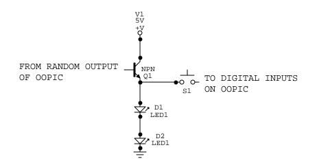
Figure 9. Schematic of Switch Circuit.
