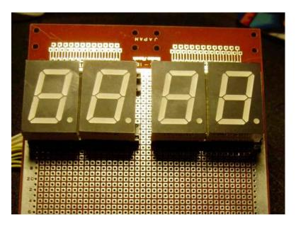
Figure 7. LED Array Used for Scoreboard and Timer.
