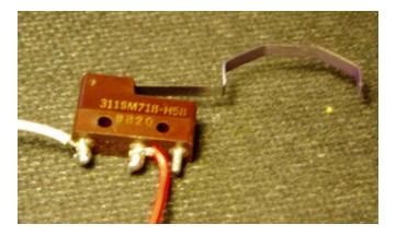
Figure 8. Single Pole-Double Throw Switch.
