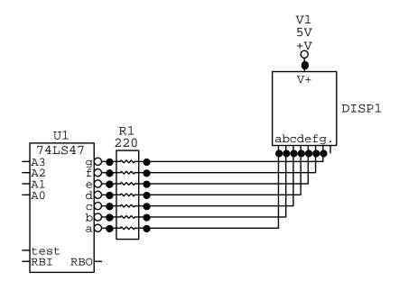
Figure 5. Schematic of Display Diver.
