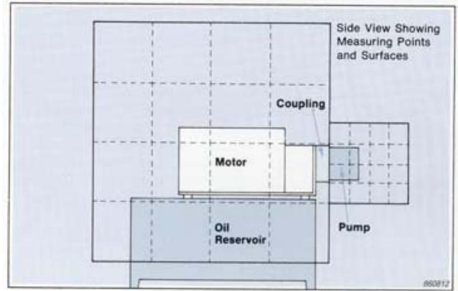
The first step in determining the sound power was to define the measurement areas. Two boxes were defined with rectangular frames and a grid of string locating the measurement points. The smaller box enclosed the pump and a larger box enclosed the motor and its oil reservoir. The boxes fitted closely around the assembly to improve the signal-to-noise ratio. In this case the "noise" consisted of the reflections from the walls of the room.
