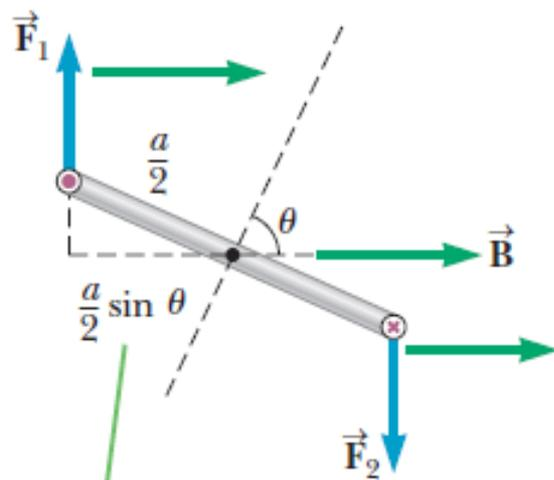
If  $\vec{B}$  is at an angle  $\theta$  with a line perpendicular to the plane of the loop, the magnitude of the torque is given by  $BIA \sin \theta$ .
