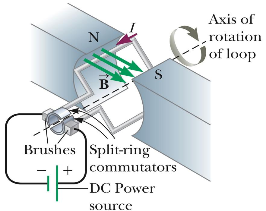
The SI unit of magnetic moment is the ampere-square meter ( $\text{A} \cdot \text{m}^2$ ). In terms of the magnetic dipole moment, the torque on the current loop is given by
