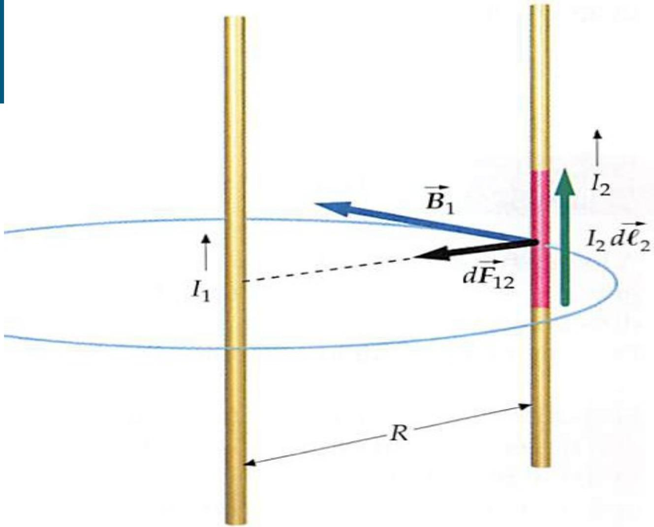
The magnitude of the magnetic force on the current element  $I_2 d\vec{\ell}_2$  is
