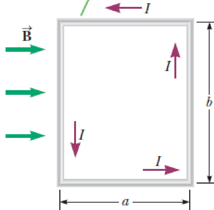
Magnetic forces act on sides with current perpendicular to  $\vec{B}$  but not on sides with current parallel to  $\vec{B}$ .
