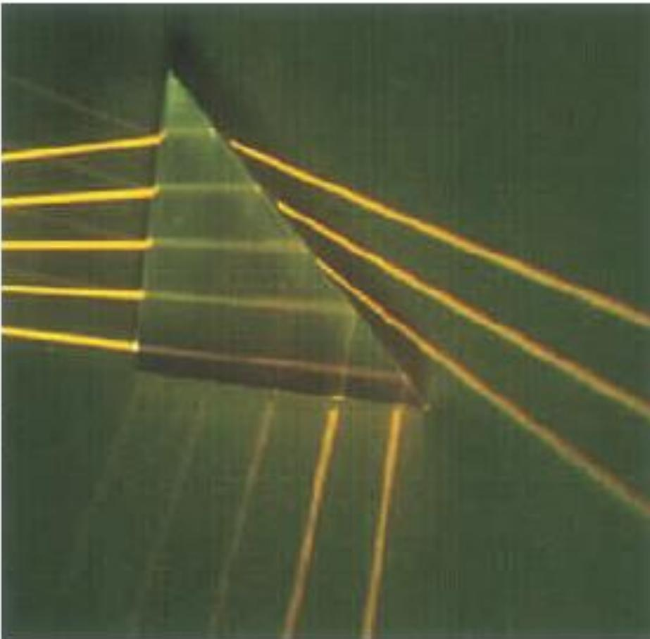
This photograph shows nonparallel light rays entering a glass prism. The bottom two rays undergo total internal reflection at the longest side of the prism. The top three rays are refracted at the longest side as they leave the prism.
