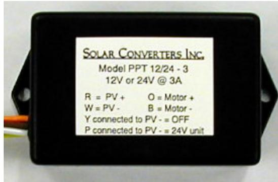
Figure 24: Solar Converters Inc MPPT
