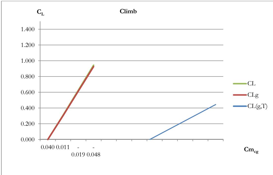
Figure 32: Power and Ground effect on pitching moment curve for climb
