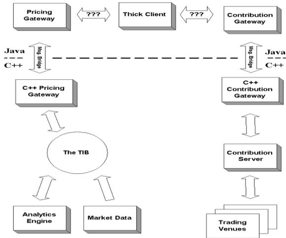
Fig 1: shows the current system design. This application pattern contains Gateways and components used in system. Channel Adapters and non-messaging protocol was used to implement Message translator. Two messaging systems are connected using Channel Adapters.[4]
