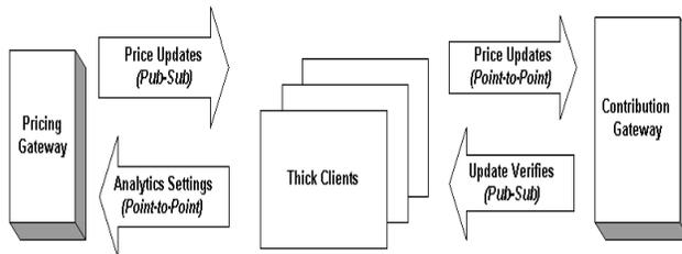
Fig 2: Message flow with Channel Types[4]
