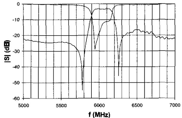
Fig. 6 – Measured Return Loss and Rejection of the YBCO/MgO multilayer filter at 77K (LN).
