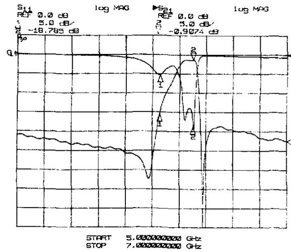
Fig. 7 – Measured Return Loss and Rejection of the YBCO/MgO multilayer filter at 77K vacuum.
