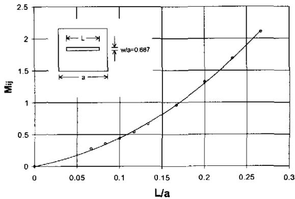
Fig. 4 – Normalized coupling coefficient as a function of the length of a slot iris, calculated by a commercial FDTD em simulator.
