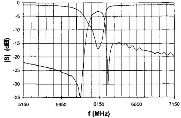
Fig. 5 – Measured Return Loss and Rejection of the Au/MgO multilayer test filter at room temp.
