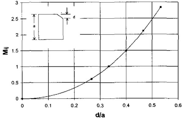
Fig. 3 – Normalized coupling coefficient as a function of the size of a corner-cut, calculated by a commercial FDTD em simulator.
