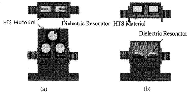
Fig. 3. Sketches of single mode, dielectric/HTS resonator filters including: (a) post resonator and (b) half-cut resonator.
