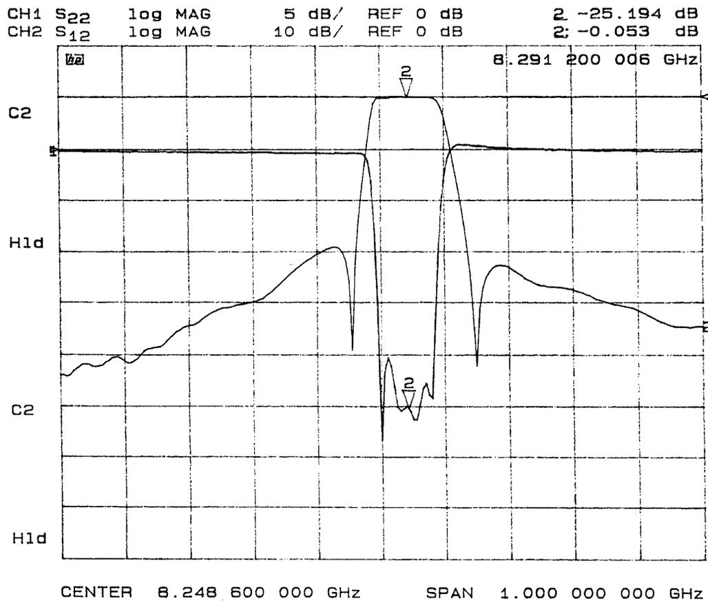
Fig. 11. Measured rejection and return loss performance of the HTSSE-II filter illustrated in Fig. 10.
