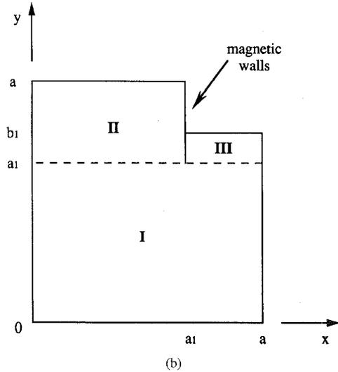
Fig. 8. Modeling of dual mode planar filters is illustrated. (a) Cut away corner section is modeled as a series of  $N$  steps. (b)  $N = 1$  step.
