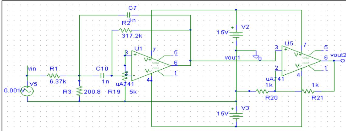
Figure 3.5. PSpice schematic of each band-pass filter.
