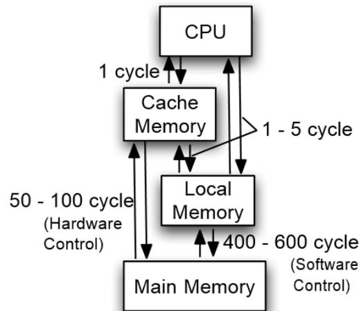
Figure 3. Core configuration and data Read/Write speeds
