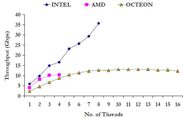
Figure 7. Throughput in Gbps of end-to-end network data transfer across number of threads for different SUTs
