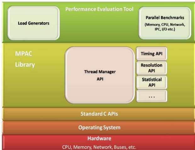
**Figure 4. A high-level architecture of MPAC Library’s extensible benchmarking infrastructure.**
