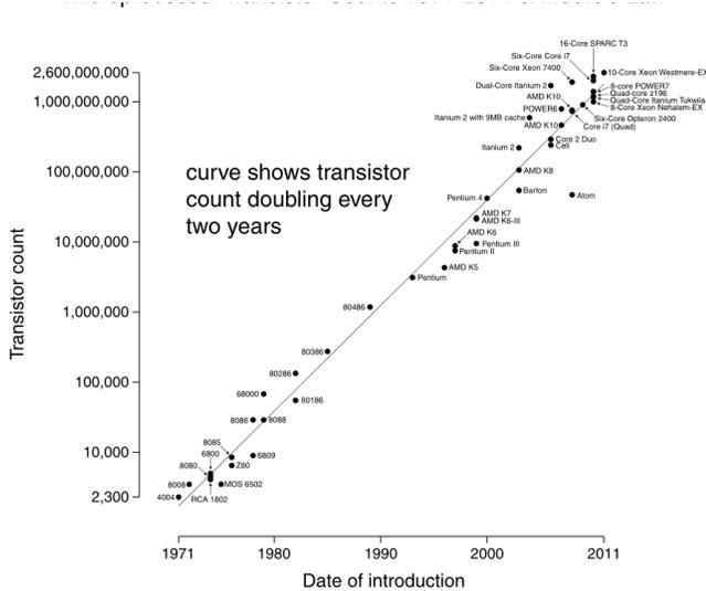
Figure 1. Microprocessor Transistor Counts & Moore's Law
