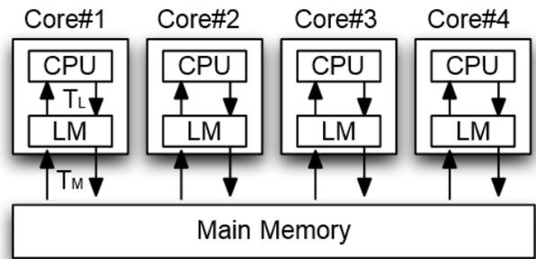
Figure 2. Basic Configuration of multi-core processor
