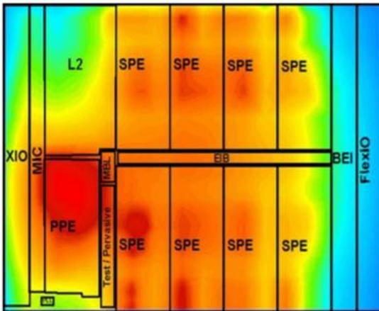
Figure 8 CELL Thermal Diagram
