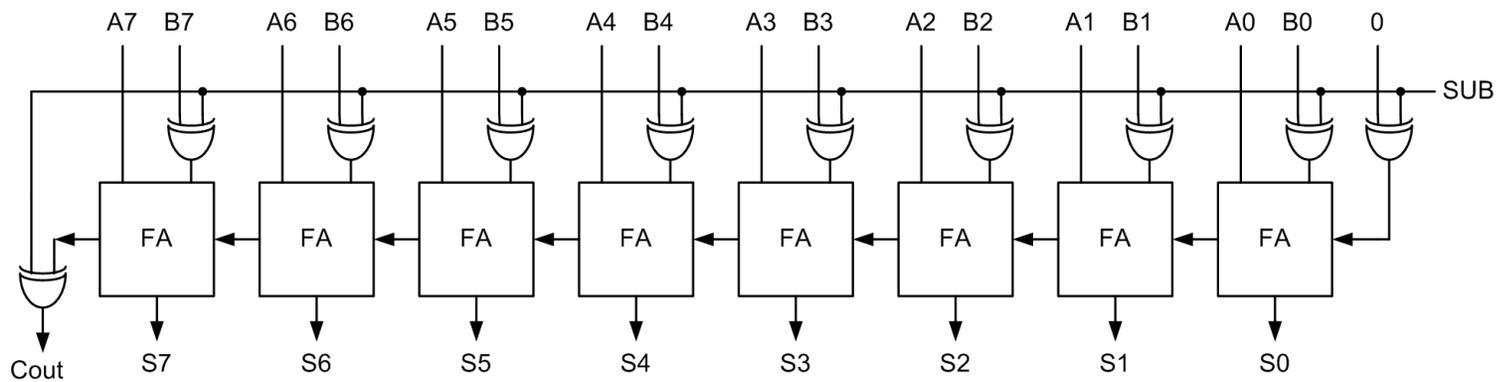
**8-bit Ripple Carry Adder Architecture**
