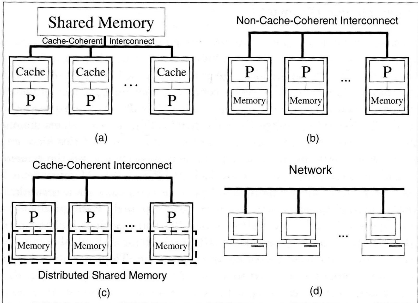
Figure 1.2: **Distributed- and shared-memory computers** – The machine (a) has physically shared memory, whereas the others have distributed memory. However the memory in (c) is accessible to all processors.
