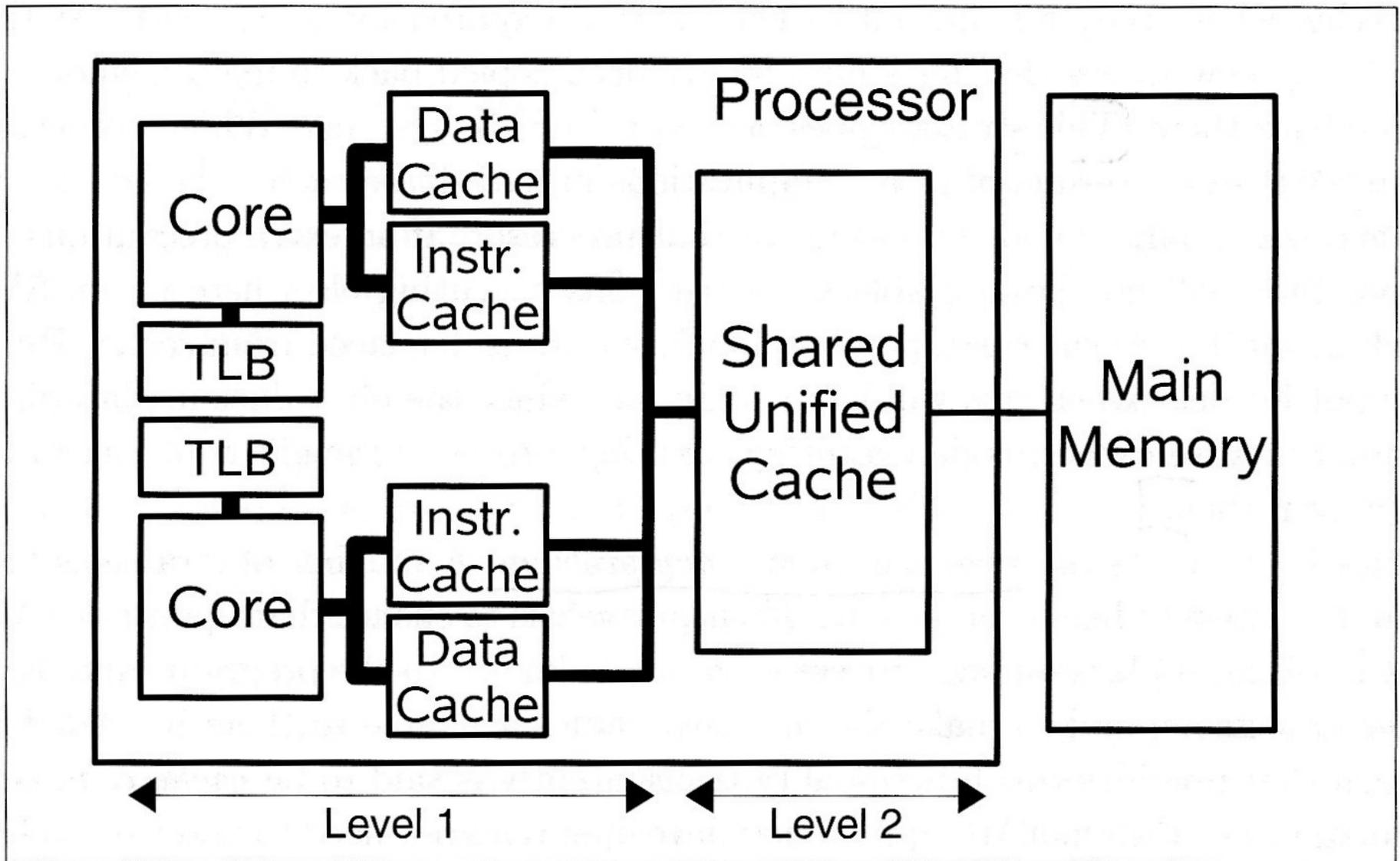
Figure 1.1: **Block diagram of a generic, cache-based dual core processor** – In this imaginary processor, there are two levels of cache. Those closest to the core are called “level 1.” The higher the level, the farther away from the CPU (measured in access time) the cache is. The level-1 cache is private to the core, but the cache at the second level is shared. Both cores can use it to store and retrieve instructions, as well as data.
