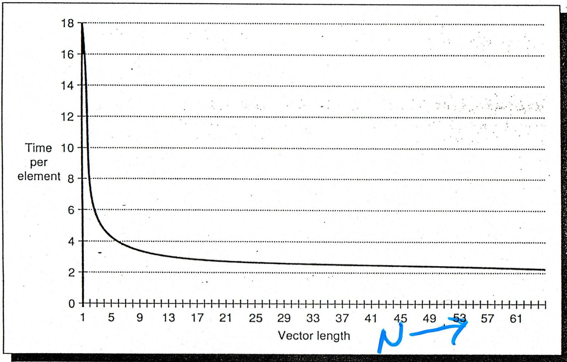
**FIGURE 7.9** The impact of just the vector start-up cost on a loop consisting of a vector assignment. For short vectors, the impact of the 16-cycle start-up cost is enormous, decreasing performance by up to nine times. The strip-mining overhead has not
