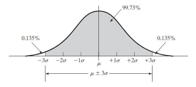
Normal distribution of process output variable, showing the  $\pm 3\sigma$  limits
