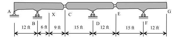
The beam shown is pin supported at point A; roller supported at points B, D, and F (note that roller supports resist movement both up and down); and has internal hinges at points C and E.
