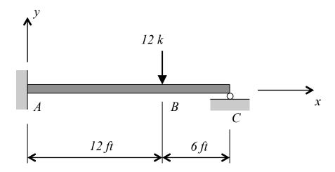
The beam analyzed by the direct stiffness method in Lab #11 is statically indeterminate to the first degree. Recall that the beam has the following properties:
