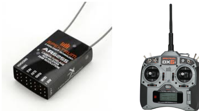
Figure 3.4: 6 channel receiver and transmitter from Spektrum
