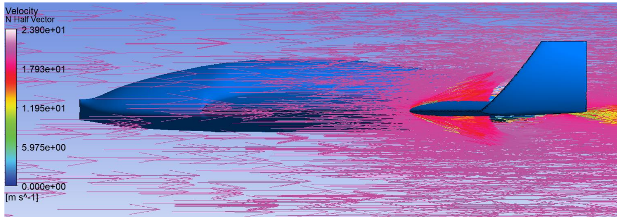
Figure 10.16 – Airflow side view (0.5 m from center plane) (72 km/h)
