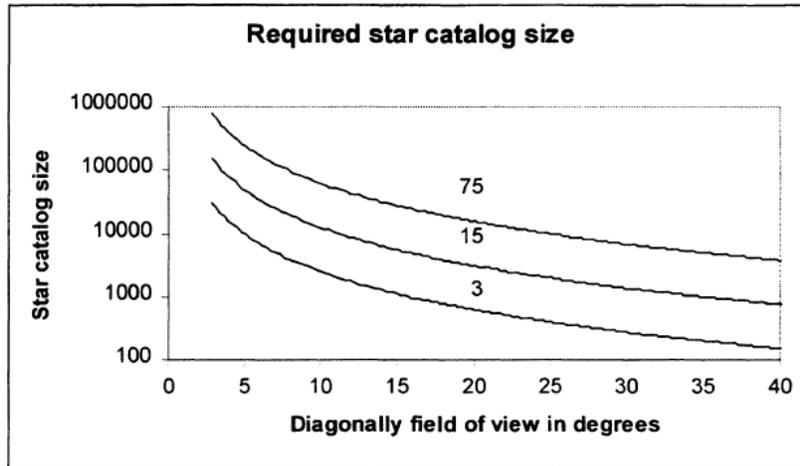
Figure 1-3: Star catalog size vs diagonal FOV [3].
