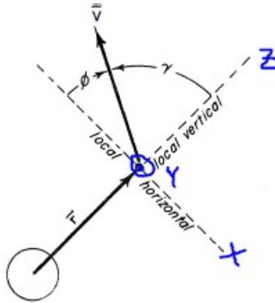
Figure 4-7: Local Vertical Local Horizontal spacecraft reference frame [10]
