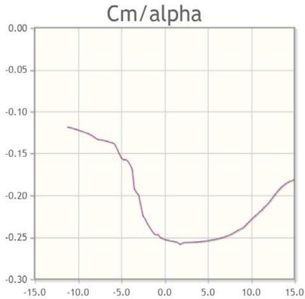
Figure 4: Coefficient of Moment vs. Angle of Attack
