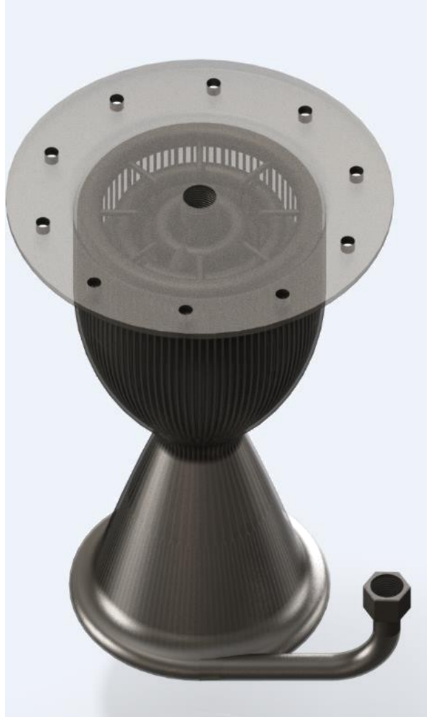
Figure 30c: 3D CAD Model of the Leon 1 Rocket Engine
