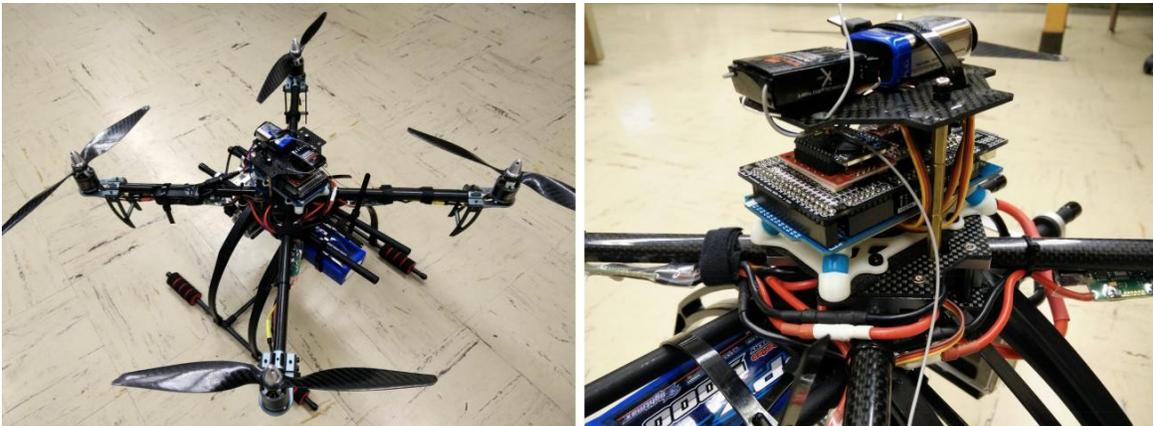
Figure 3. Assembled quadcopter testbed.
