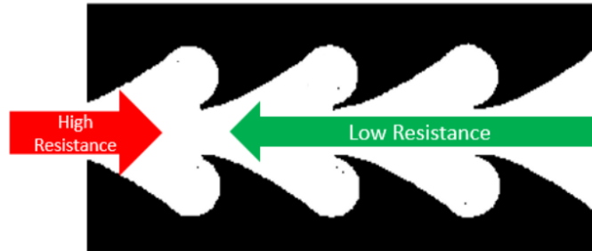
Figure 3.8: Fluidic diode showing high resistance to flow in one direction, and low resistance to flow the other direction [12].
