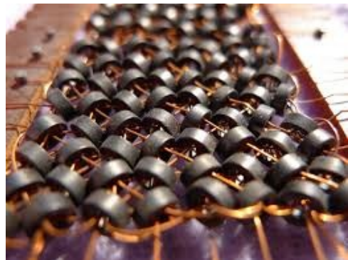
Figure 1. Iron core rope memory
