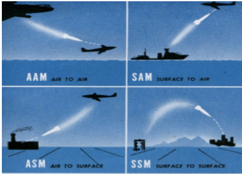
Figure 1.1 - Demonstration of missile classification [7].
