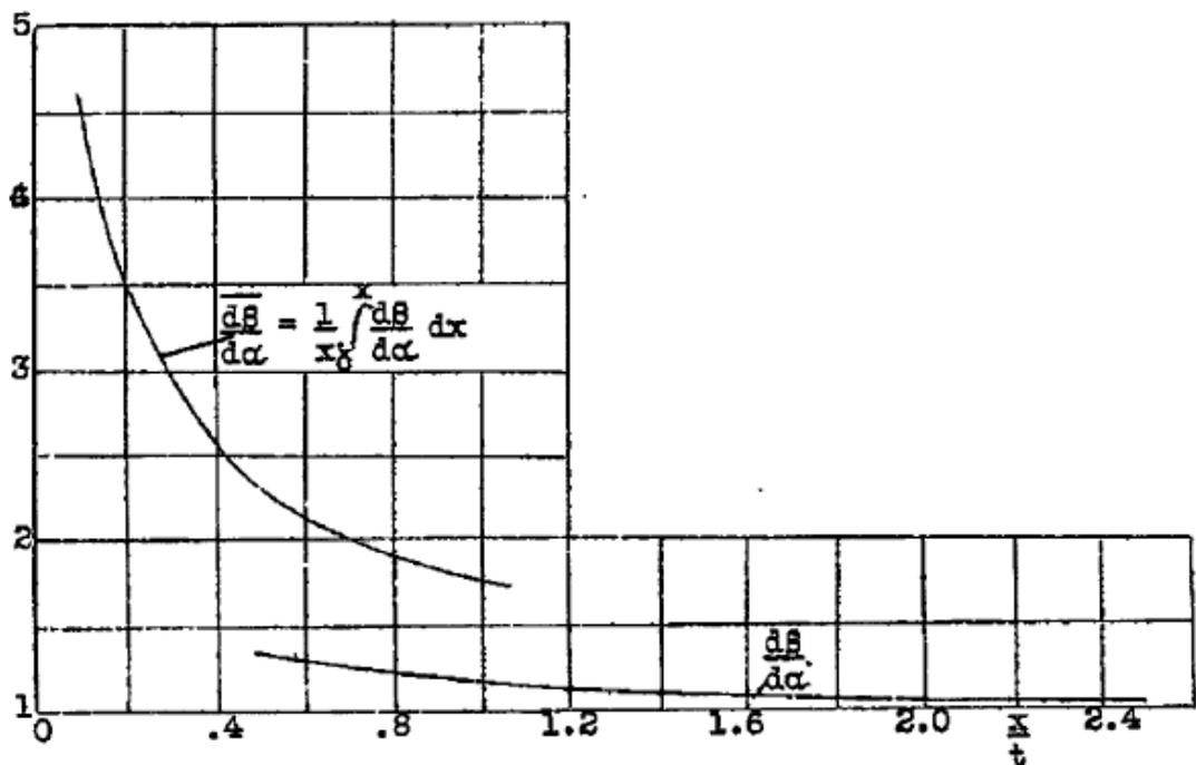
**Figure 9: Normal values for upwash ahead of the wing (Multhopp, 1942)**
