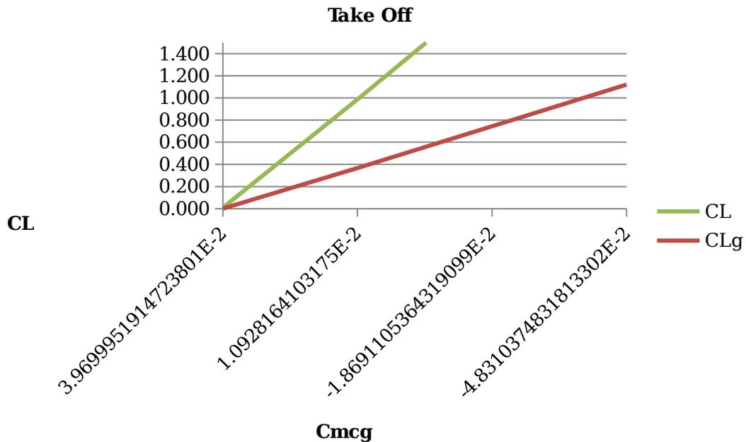
**Figure 28: Ground effect on pitching moment for take off**
