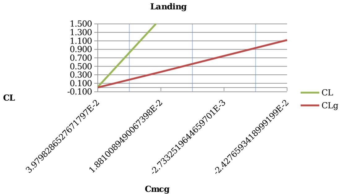
**Figure 29: Ground effect on pitching moment for landing**
