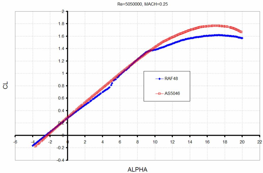
**Figure 12: CL- $\alpha$  Curve Comparison - plotted with *Xfoil* (Nordin, 2006)**
