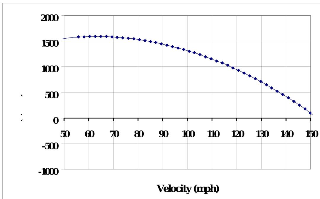
**Figure 21: Rate of Climb vs. Velocity, 6000 Ft. Density Altitude (Nordin, 2006)**
