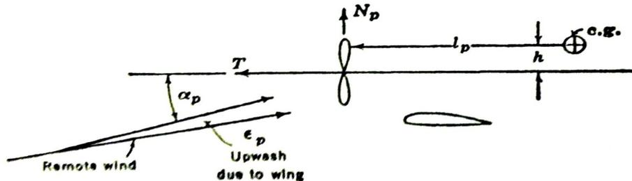
**Figure 11: Direct forces cause by propeller (Perkins & Hage, 1949)**
