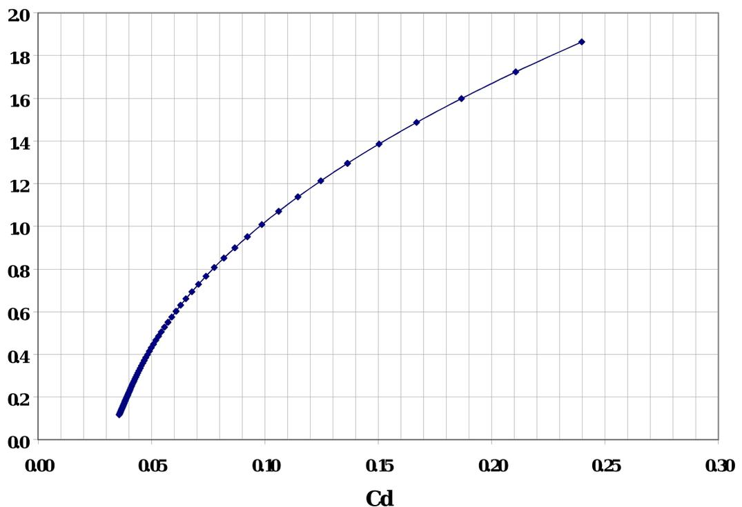
**Figure 20: Drag Polar for Modified KR-2 at Gross Weight and at Density Altitude of 6000 Feet (Nordin, 2006)**
