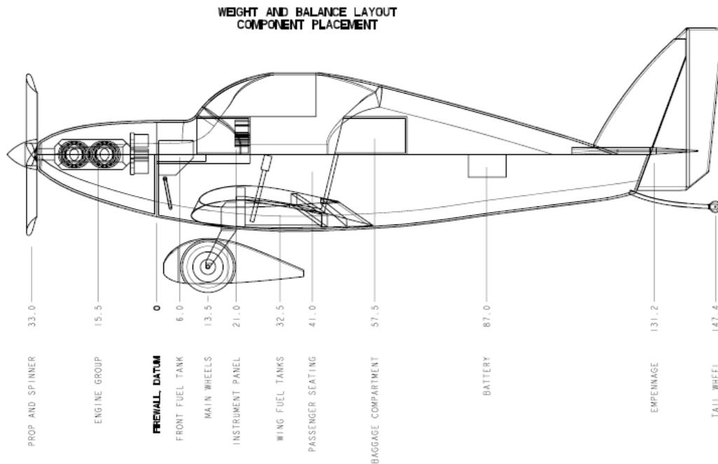
**Figure 23: Locations of Major Components for Weight and Balance
