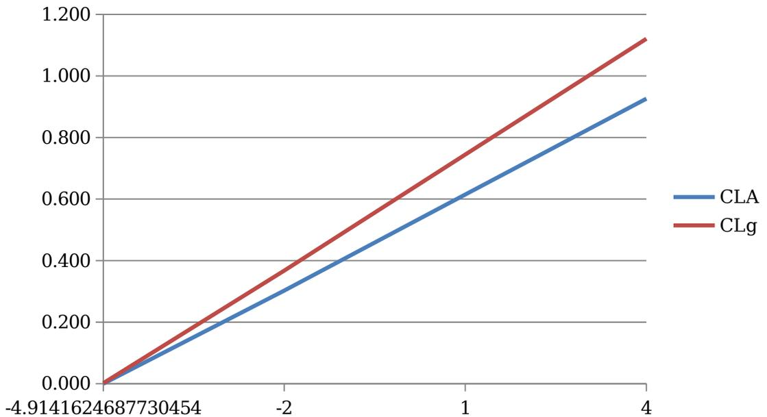
**Figure 26: Ground effect on lift at take off**
