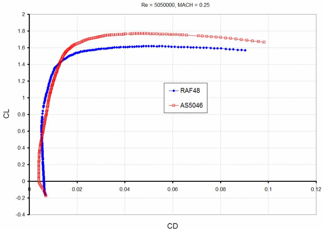
**Figure 13: Drag Polar Comparison - plotted with *Xfoil* (Nordin, 2006)**
