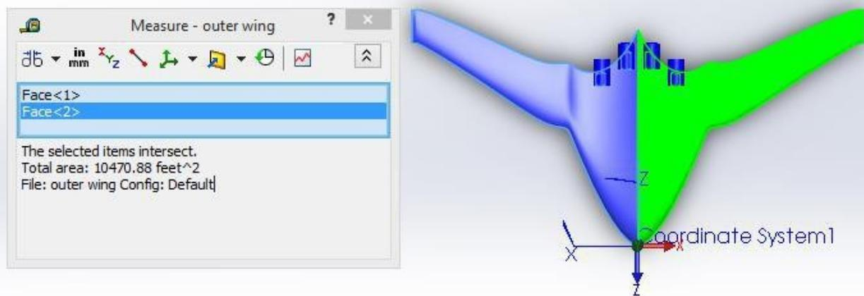
Figure 44: Measurement of wet area of wing + center body from solid work model
