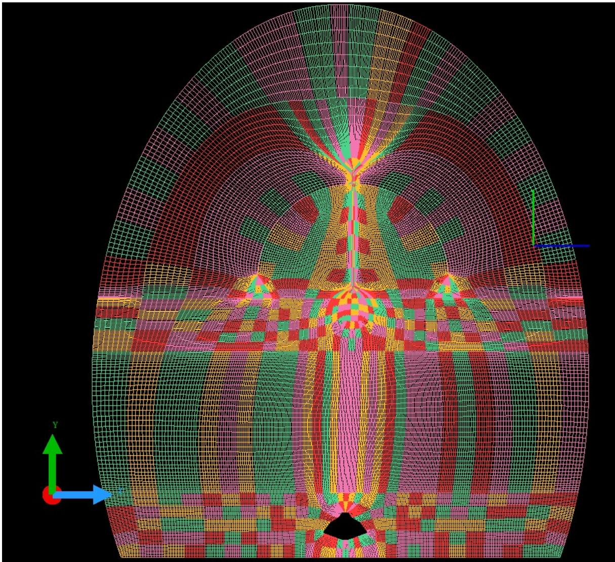
Figure 20 – Sliced front view of capsule-parachute system grid
