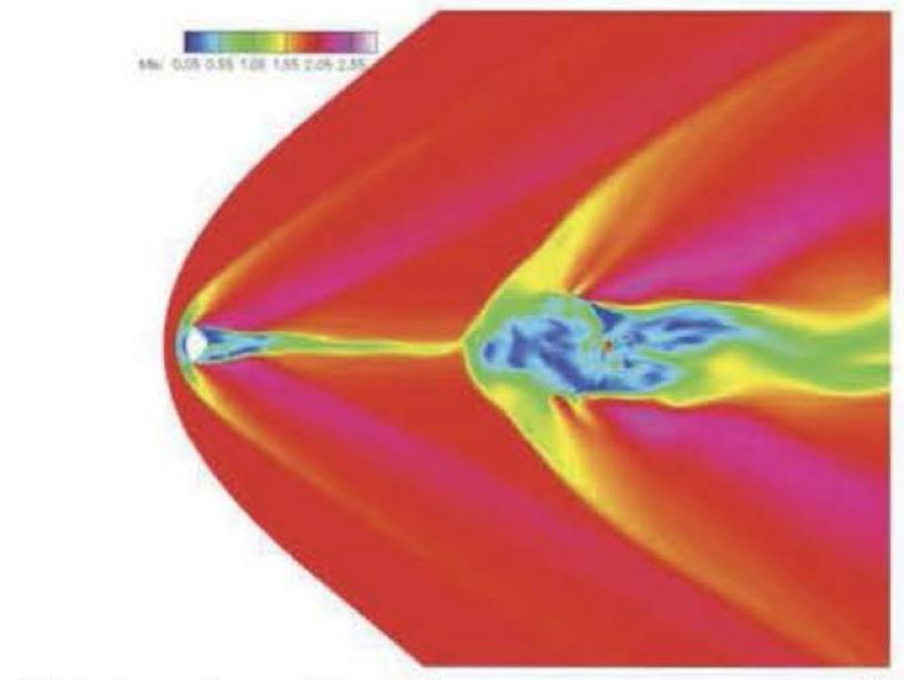
Figure 3 – Rigid Parachute CFD simulation by Sengupta et al.
