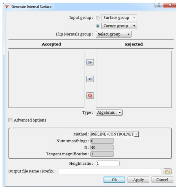
Figure 14– GridPro GUI internal surface input window
