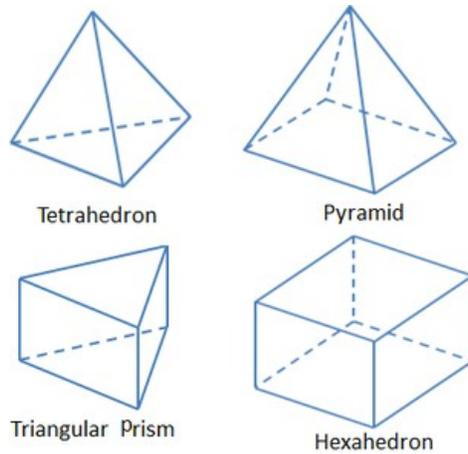
Figure 4 – Finite Volume Cell types
