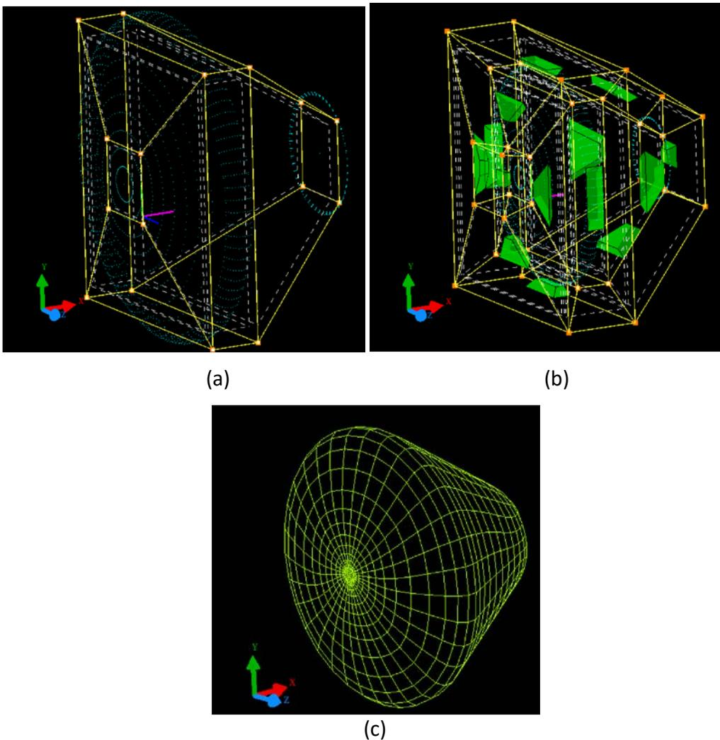
Figure 7 – GridPro Wrap tool for O-grids (a) topology at the Orion surface (b) Wrapped topology including block preview (c) Computed grid result
