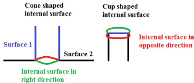
Figure 13 – Possibilities of internal surface creation
