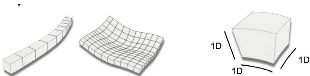
Figure 5 – Structured Mesh mapping
