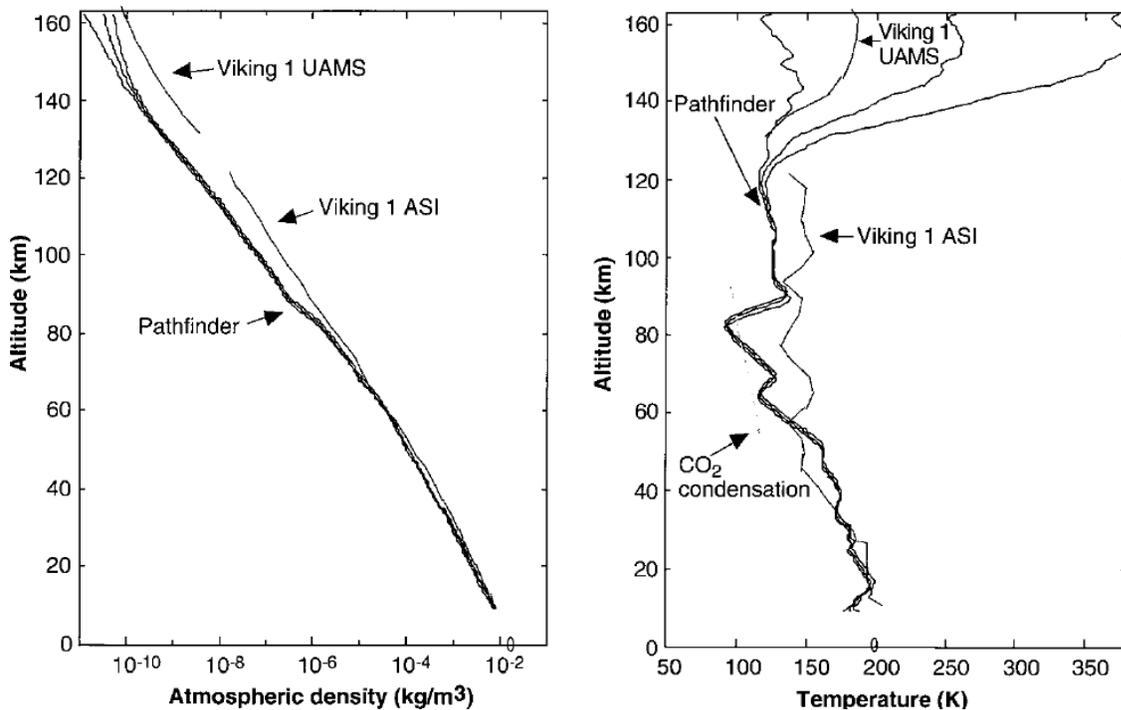
Figure 1 – Mars Atmospheric density and temperature profile
