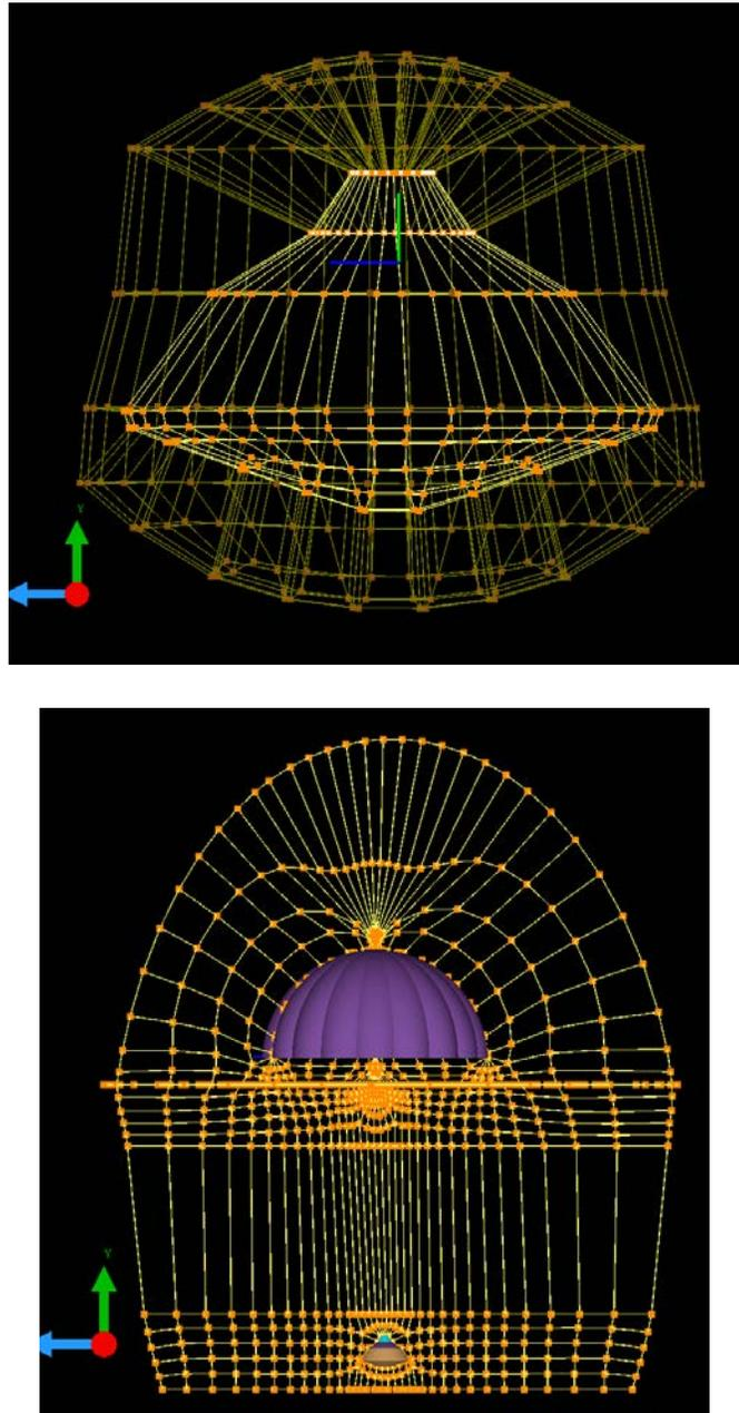
Figure 18 – Final topology (a) capsule displaying O-grid (b) topology face pattern on parachute
