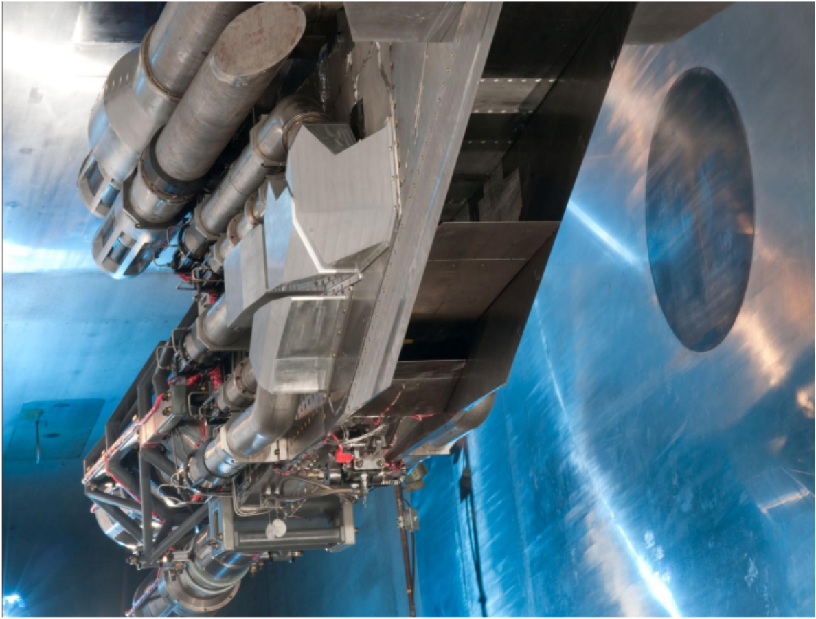
Figure 1.7. NASA combined cycle engine large scale inlet mode transition experiment (CCE LIMX) (15).
