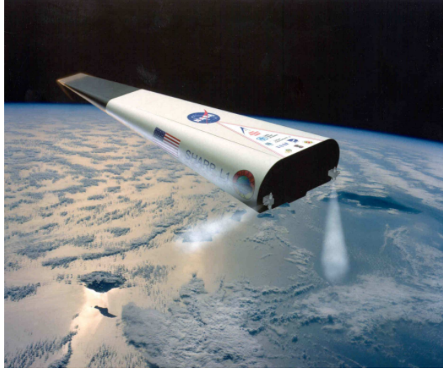
Figure 1.7: Proposed SHARP-L1 geometry with hybrid cone-wedge geometry [30].
