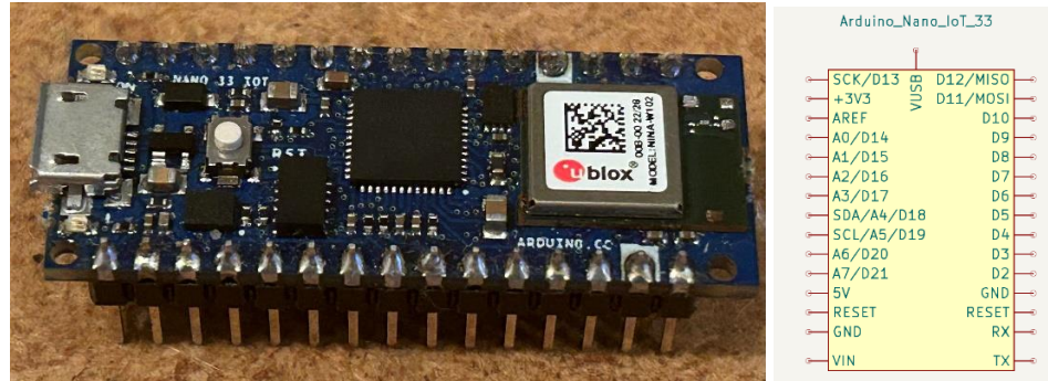
Figure 2.16. Arduino Nano IoT 33 MCU (left) and simple wiring diagram (right).
