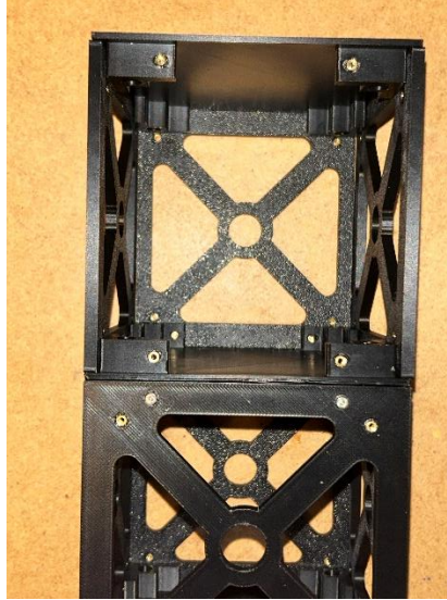
Figure 5.1. Chassis walls and baseplates thermal-screw assembly.
