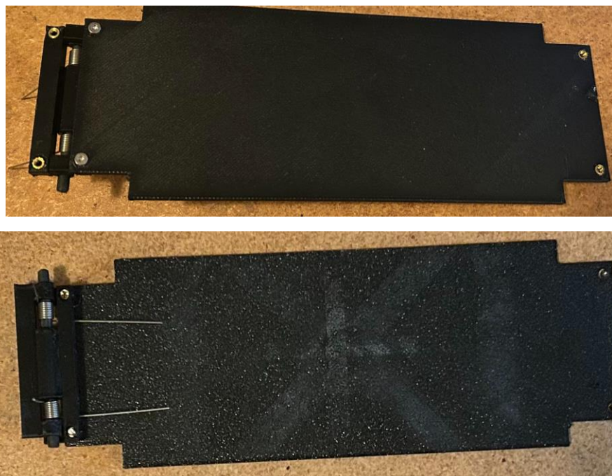
Figure 5.3. Single-set torsion spring hinge and solar panel assembly top and bottom surface, respectively.
