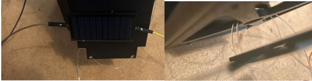
Figure 5.11. Initial fishing line insertion (left) and X-cross section wrapping (right).
