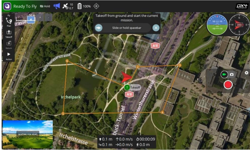
Figure 5.3: QGroundControl user interface with waypoint mission loaded onto vehicle [31].
