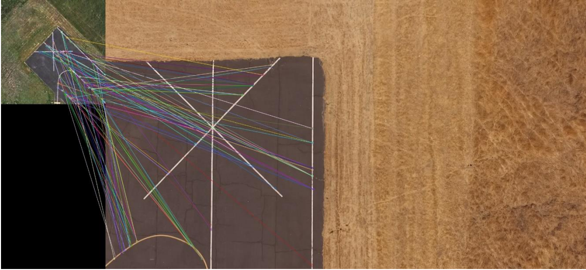
Figure 6.13: SIFT feature matching sample first waypoint between map and UAV camera stream at 25 meters.
