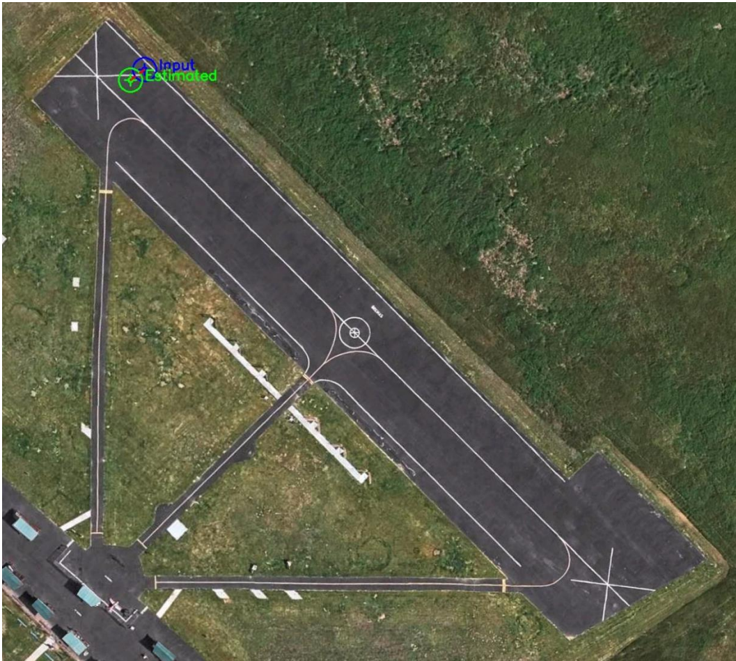
Figure 6.14: Navigation algorithm position estimate and true state of the first waypoint.
