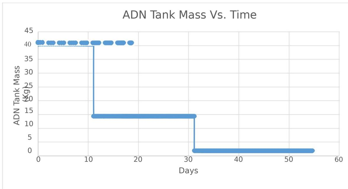
Figure 31: Time Vs. ADN Used in Scenario 2
