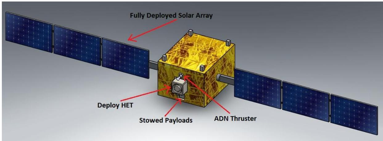
Figure 12: Isometric view of Deployed Concept Model [4]
