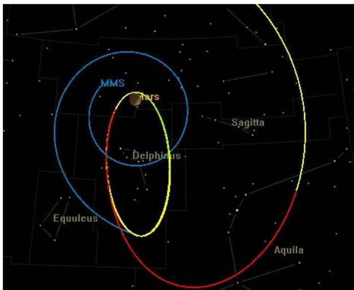
After performing the  $\Delta V$  maneuver to decrease eccentricity of the orbit, as part of Phase 5.B the HET starts firing to continue to reduce the eccentricity of the orbit and achieving a desired eccentricity and then continue to control the attitude of the satellite. The MMS can continue to adjust its orbit altitude and eccentricity using the HET onboard. The mass of the MMS and its propellant after Phase 5.B HET based maneuver will be the following.
