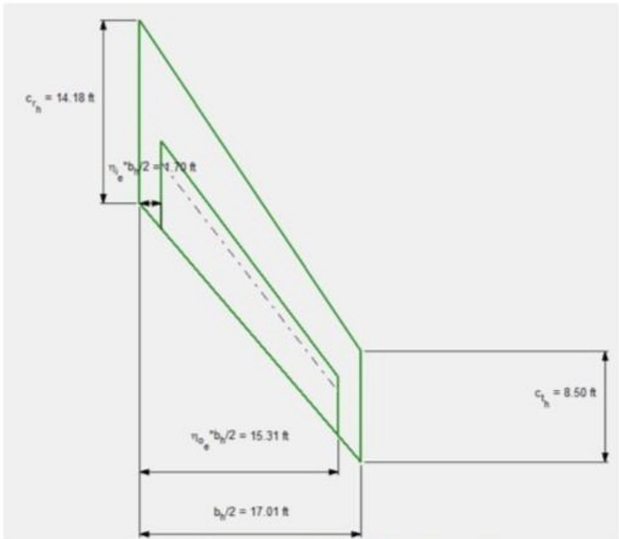
Figure 106: Elevator location and sizing obtained from AAA
