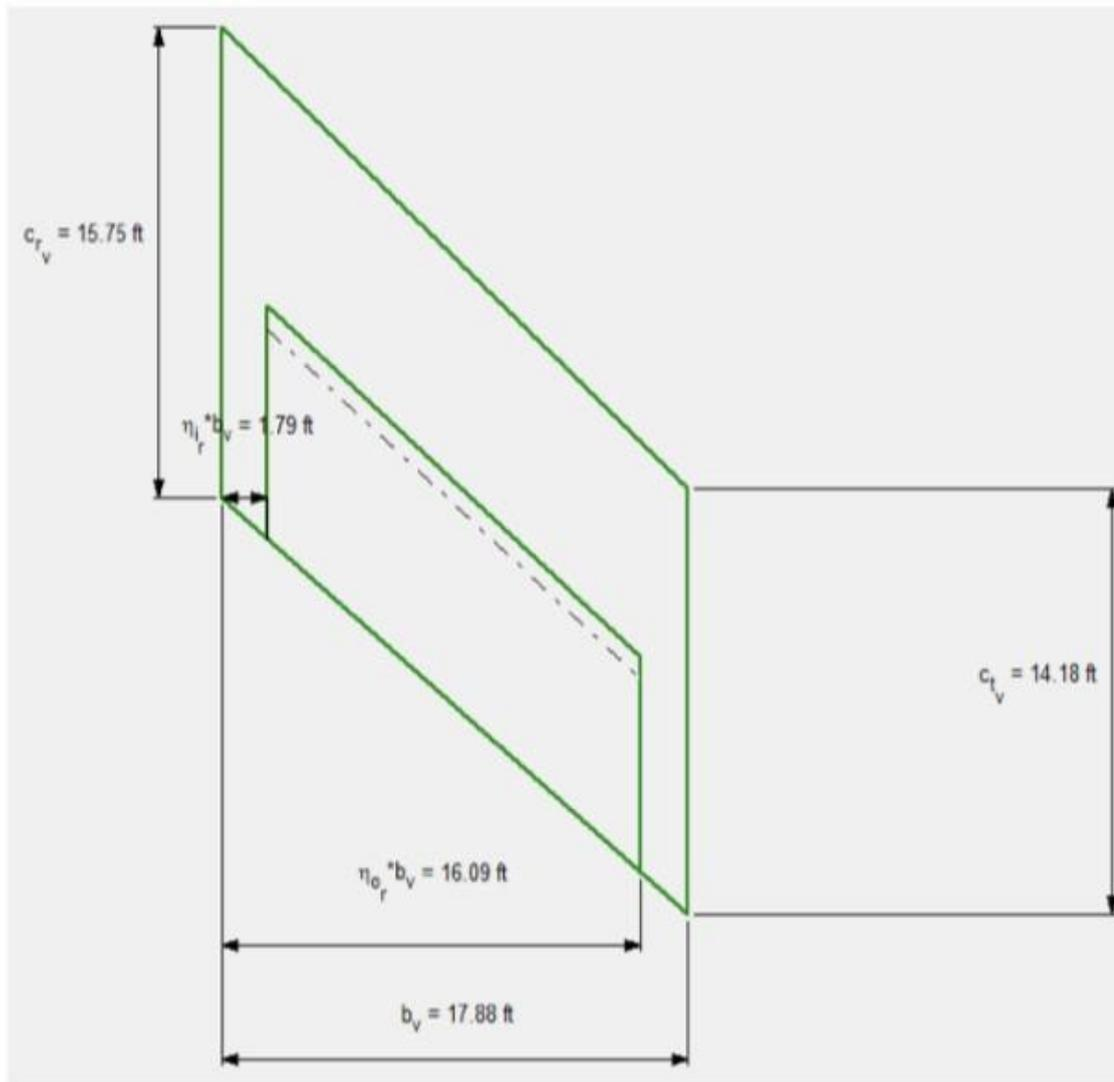
Figure 102: Rudder Location
