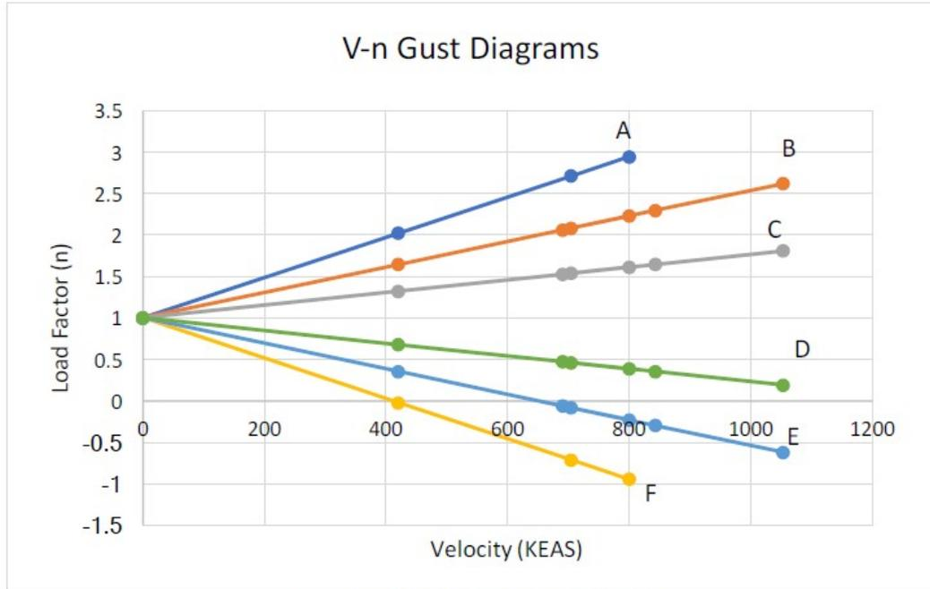
Figure 150: V-n Gust Diagram (in Knots)
