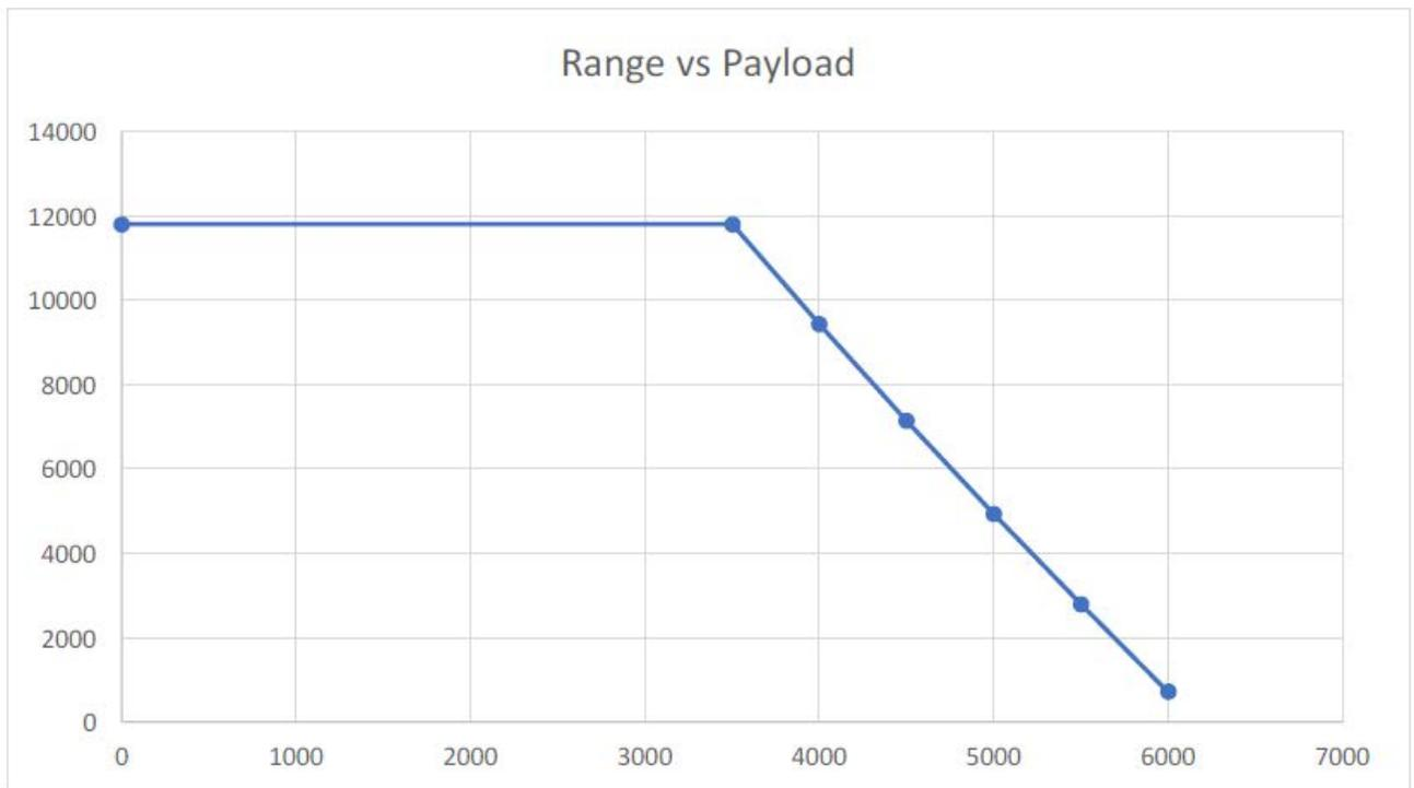
Figure 21: Trade study between the Range vs Payload
