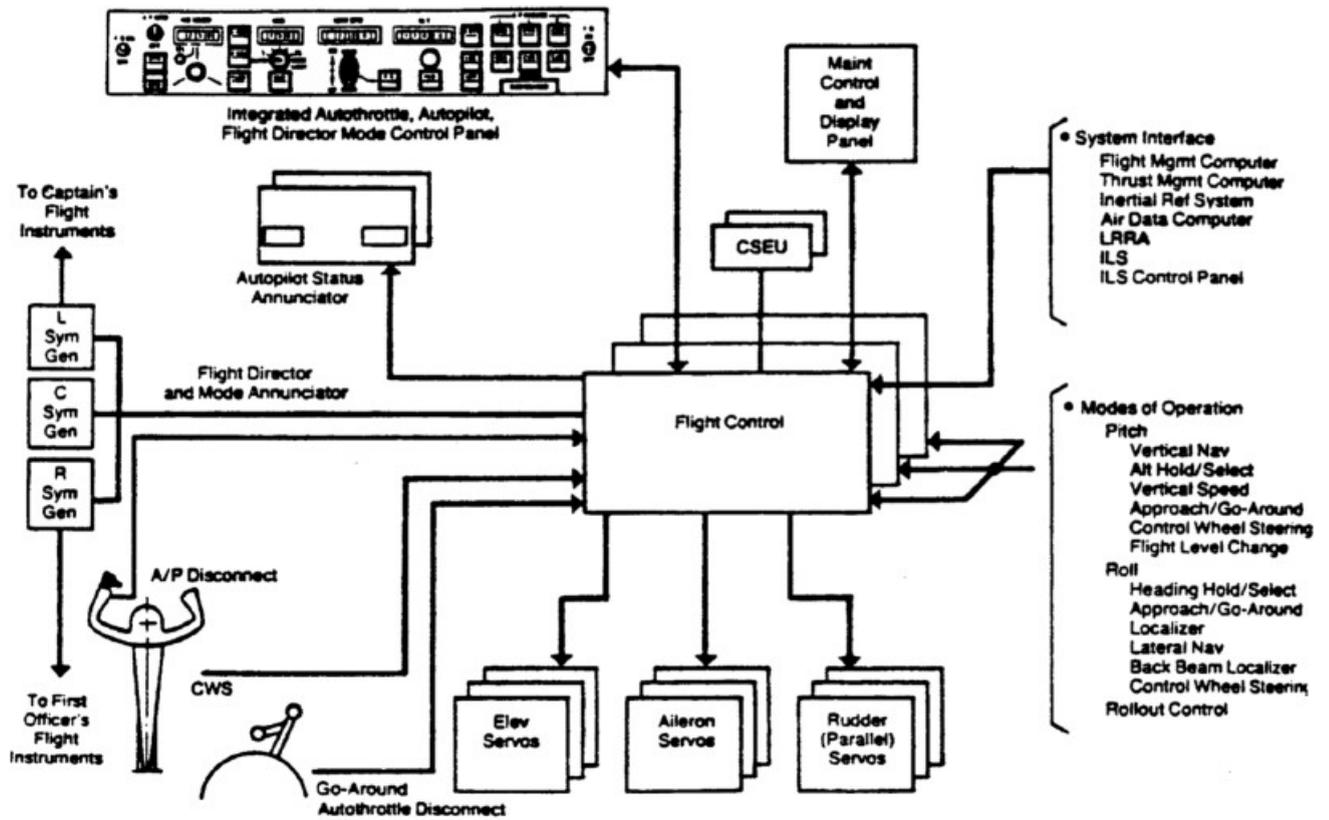
Figure 10: Flight Control Computer Functions
