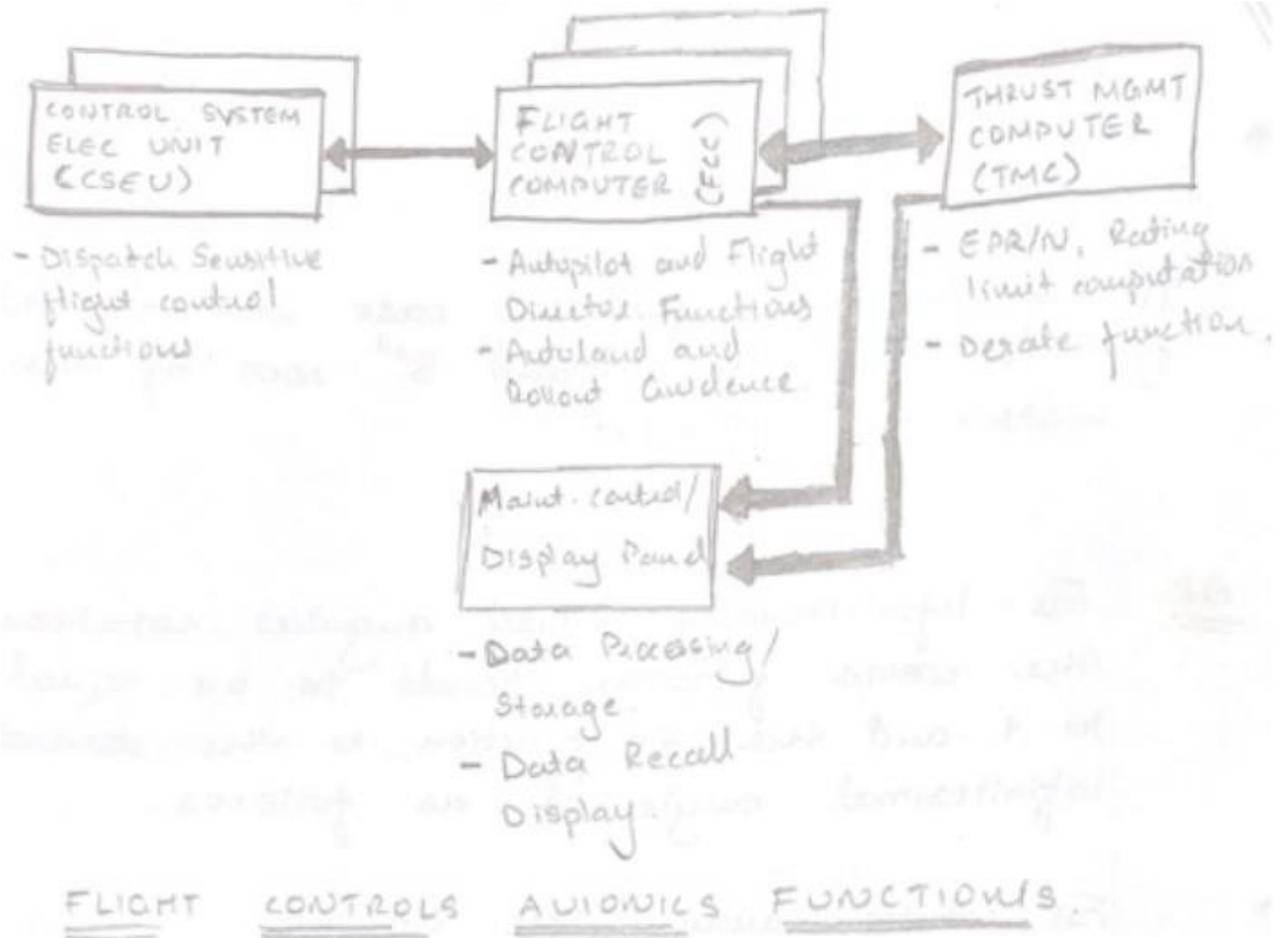
Figure 12: Flight Controls Avionics Functions
