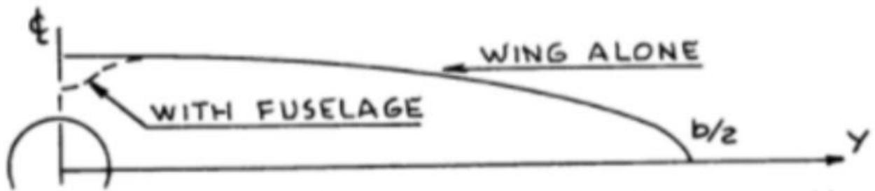
Figure 65: Effect of fuselage on wing span loading
