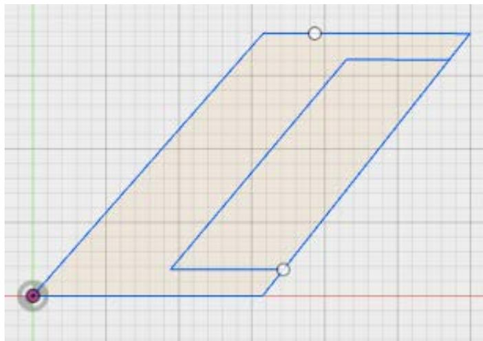
Figure 141: Side view of the vertical stabilizer
