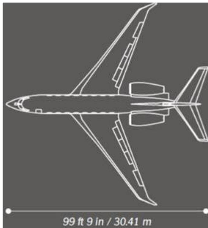
**Figure 1.4: Top view of Gulfstream G650**
