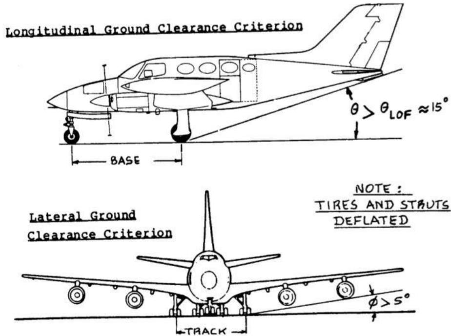
Figure 114: Longitudinal Ground Clearance Criterion
