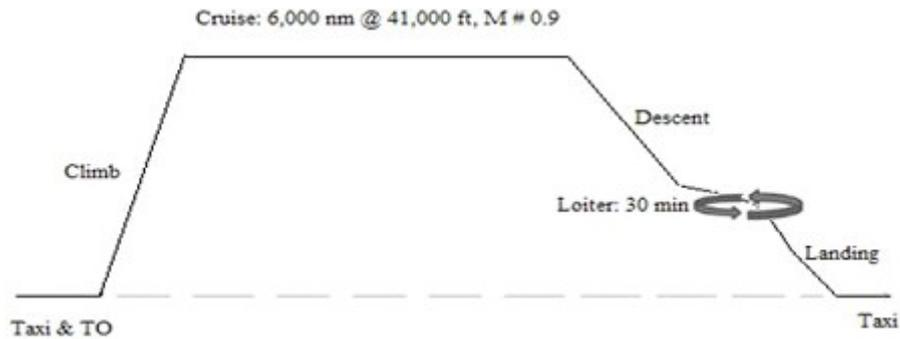
Figure 1.1: Flight mission profile of proposed aircraft
