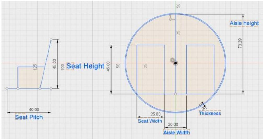
Figure 69: Cross-sectional view of the Fuselage (all units in inches)
