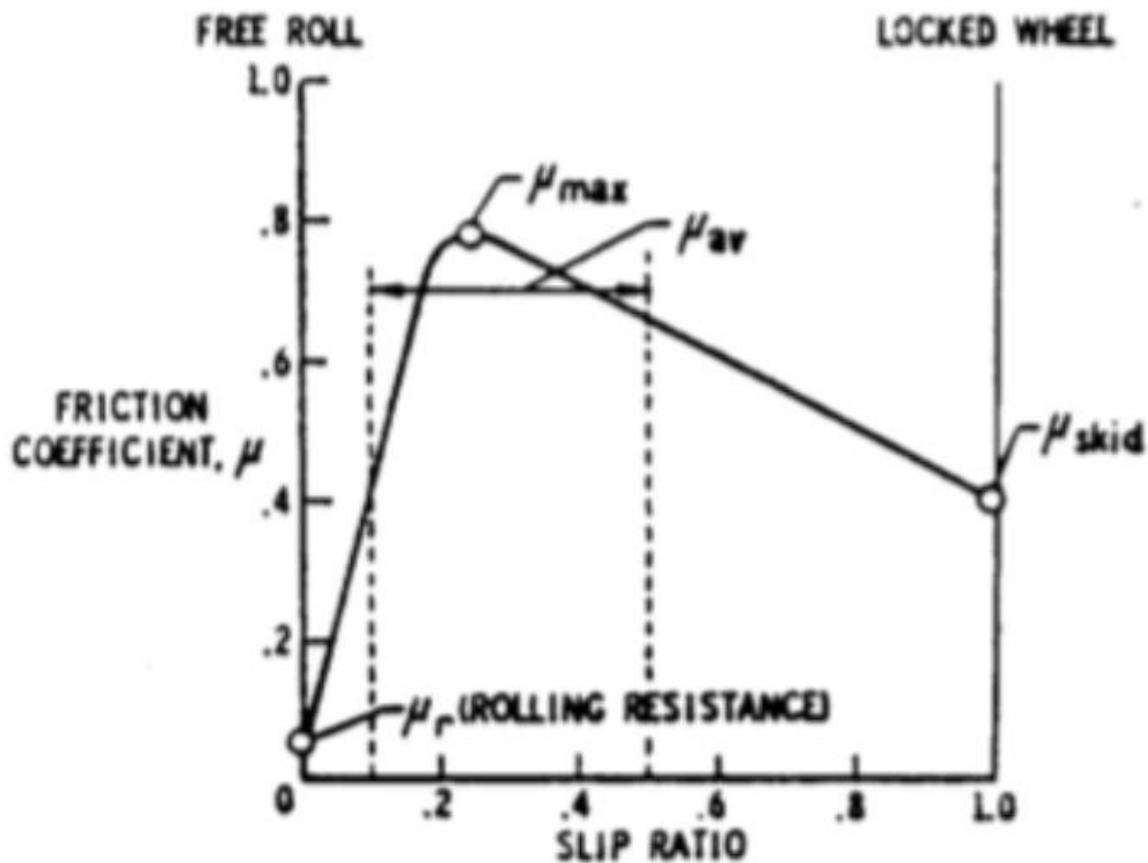
Figure 148: Effect of slip ratio on ground friction coefficient
