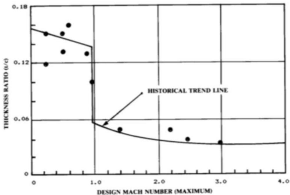
Figure 77: Design Mach number versus the thickness ratio
