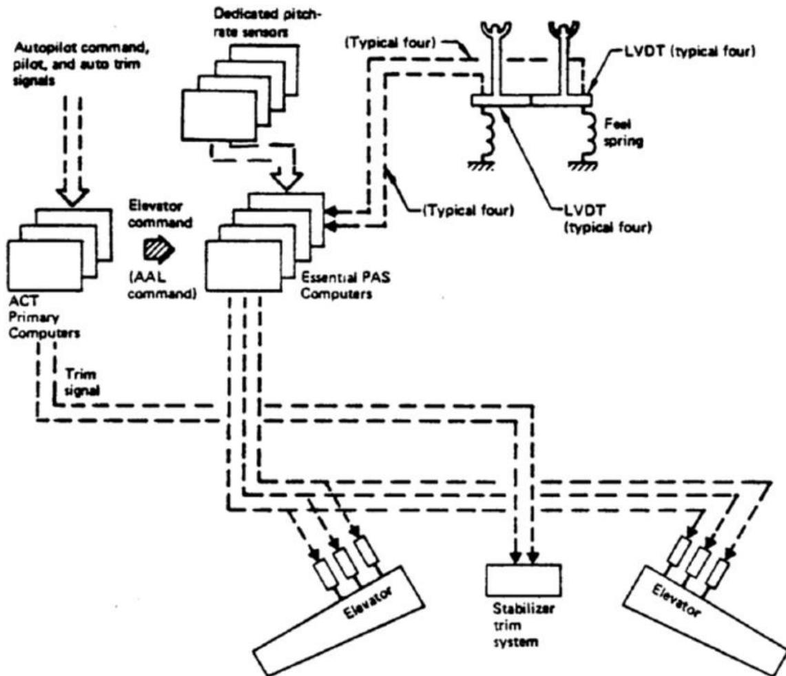
Figure 4: Fly-by-wire Hydraulic Elevator control System of the TSBJ
