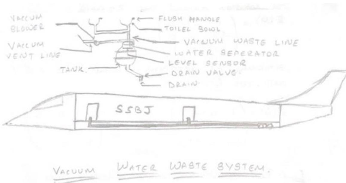
Figure 16: Vacuum Water System for the TSBJ
