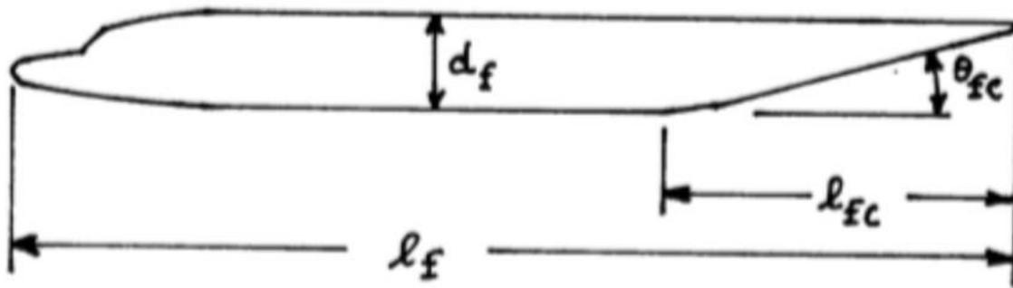
Figure 57: Dimensions of an aircraft
