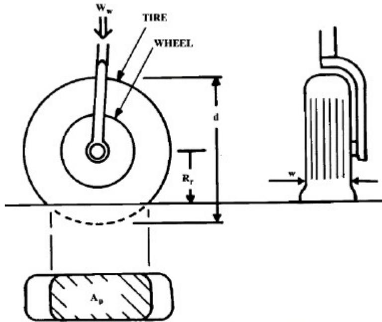
Figure 117: Tire Contact Area Definition
