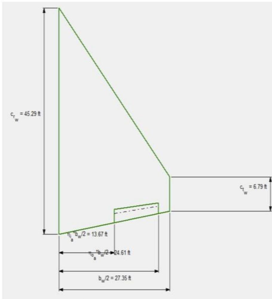
Figure 83: Aileron sizing obtained from AAA
