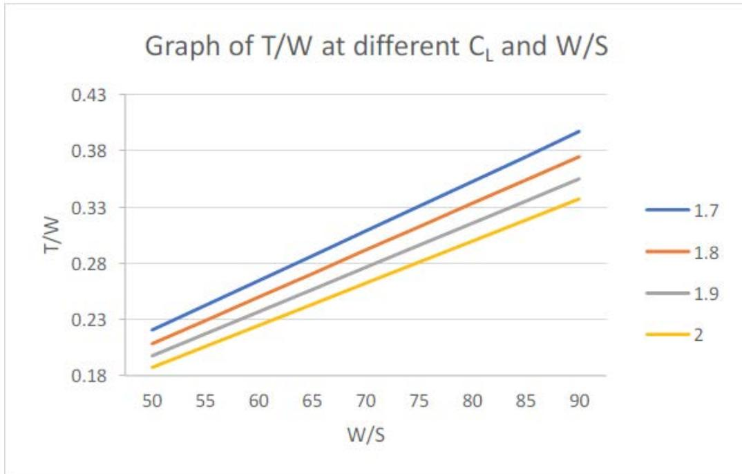
Figure 27: Graph of T/W at different C<sub>L</sub> and W/S
