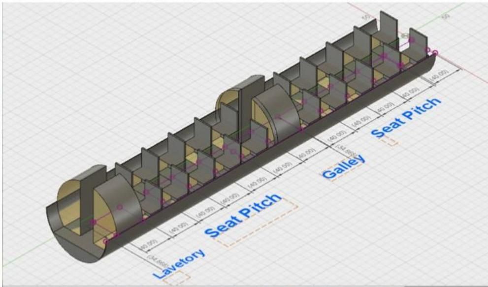
Figure 70: 3D view of the interior layout of the fuselage (all units in inches)
