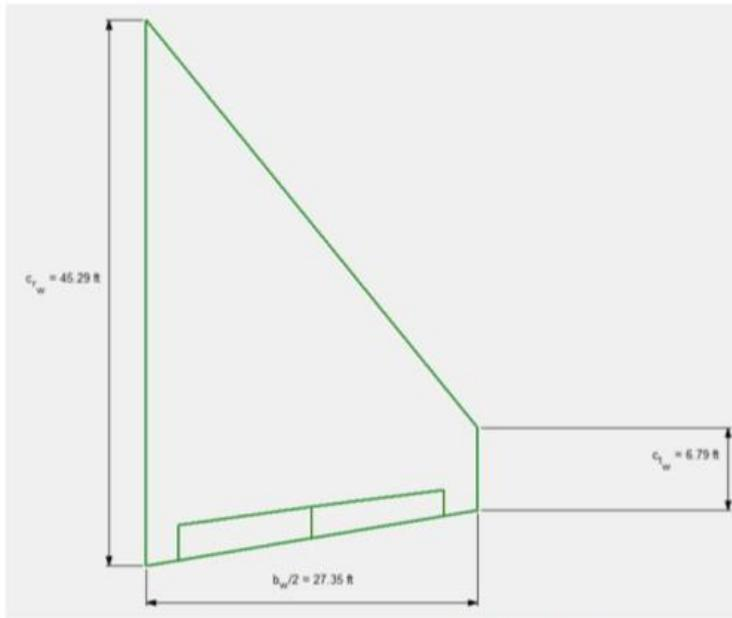
Figure 85: Aileron and Flap Locations Obtained from AAA
