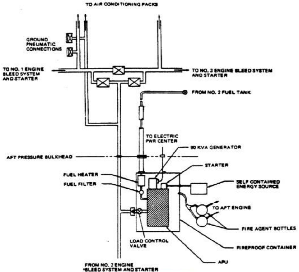
Figure 7: APU electrical system layout
