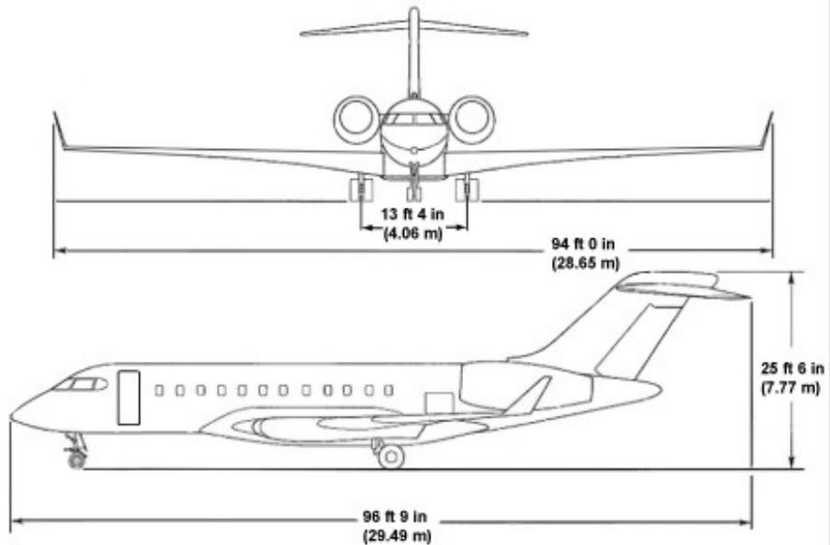
**Figure 1.6: Bombardier Global 5000 Three Views Drawing**
