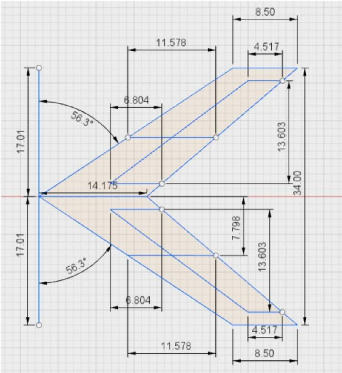
Figure 108: Elevators and horizontal stabilizer dimensions (all dimensions in fts)
