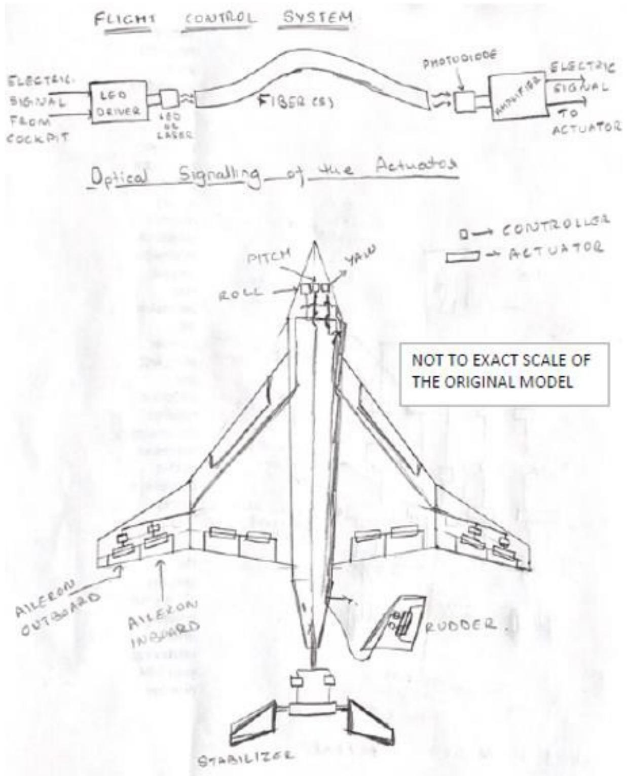
Figure 1: Electro-Mechanical Flight Control System of the TSBJ
