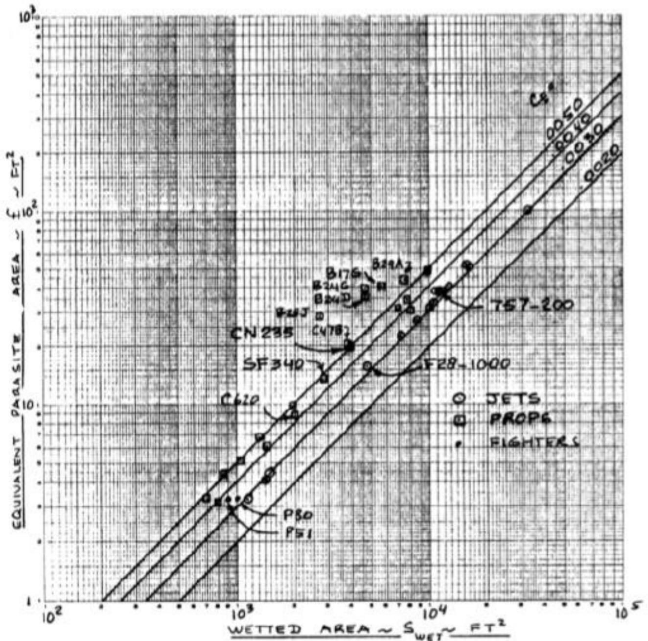
Figure 34: Relation between the wetted area and the equivalent parasite area
