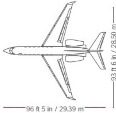
**Figure 1.2: Gulfstream G550 Three View Drawing**
