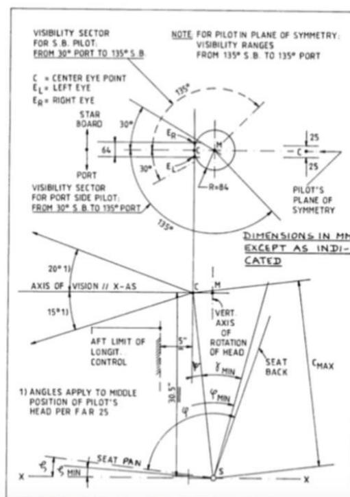
Figure 50: Visibility requirements for the port and starboard side.
