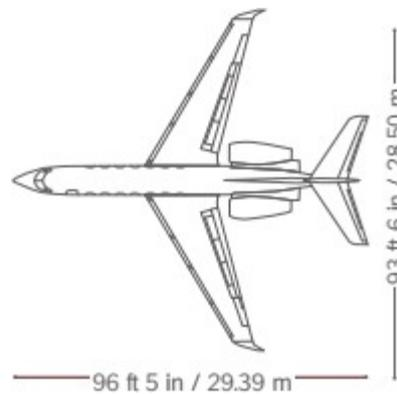
**Figure 2.1: Gulfstream G550 Three View Drawing**
