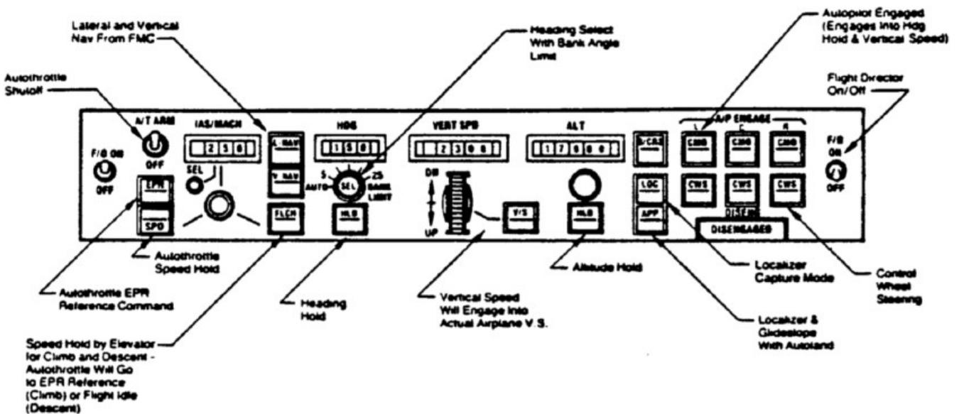
Figure 11: Autopilot/Auto throttle Control Panel
