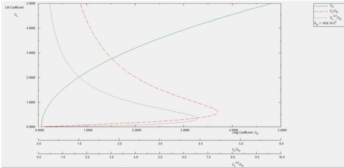
Figure 130: CL vs CD plots for take-off flaps-gear down configuration
