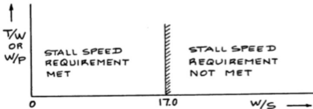
Figure 23: Example of the Stall speed sizing
