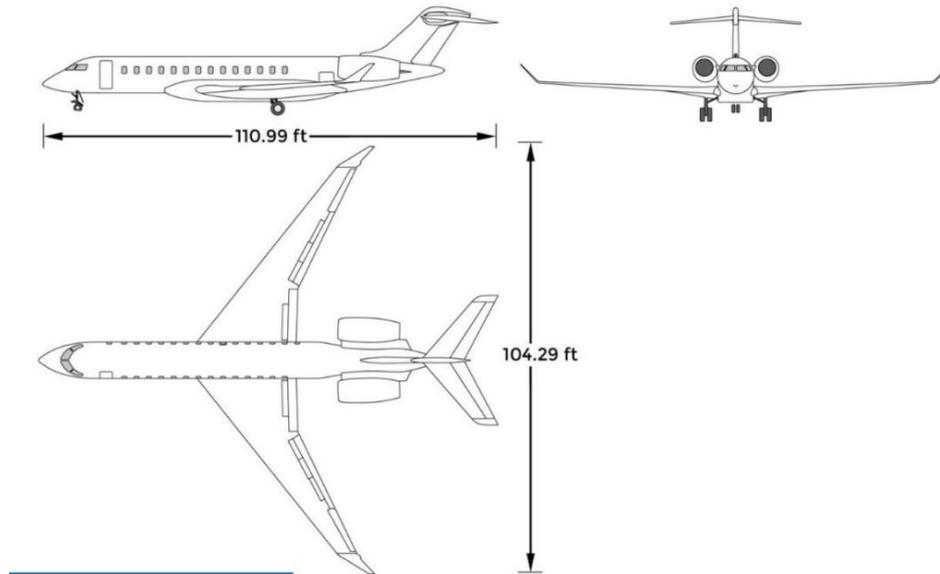
**Figure 1.8: Bombardier Global 7000 Three Views Drawing**
