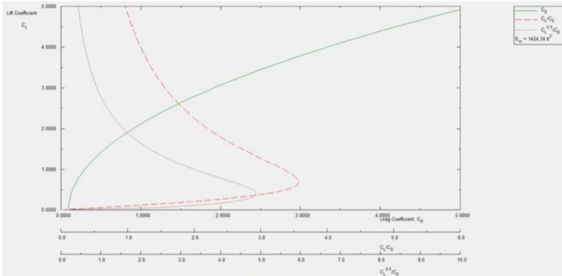
Figure 134: CL v/s CD plots for Landing-Flaps gear up configuration
