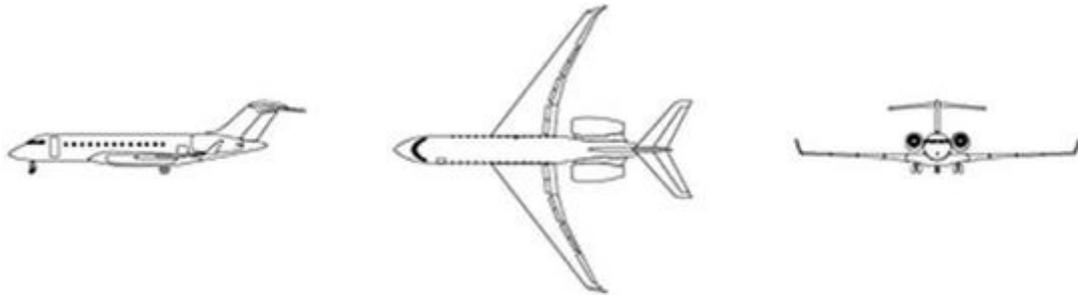
**Figure 2.6: Bombardier Global 6000 Three View Drawing**
