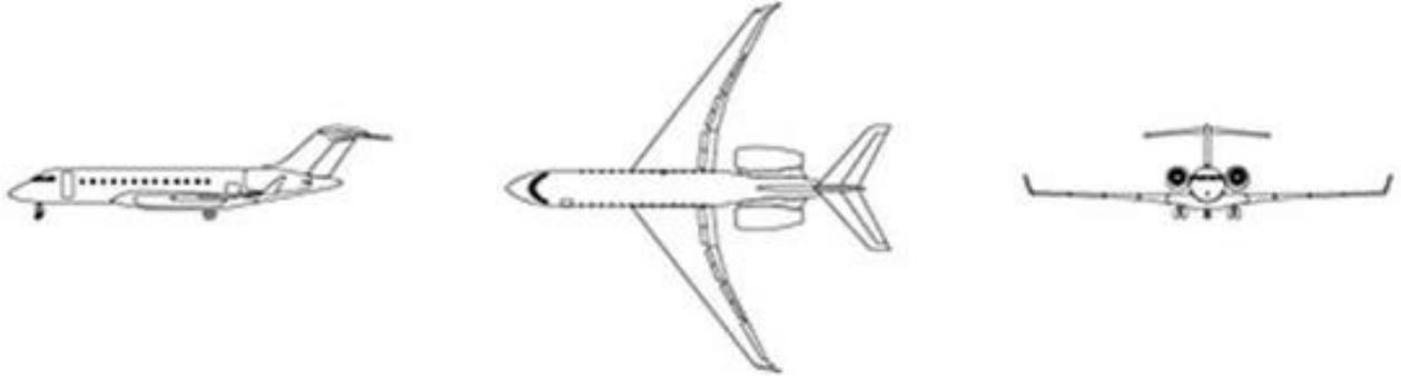
**Figure 1.7: Bombardier Global 6000 Three Views Drawing**
