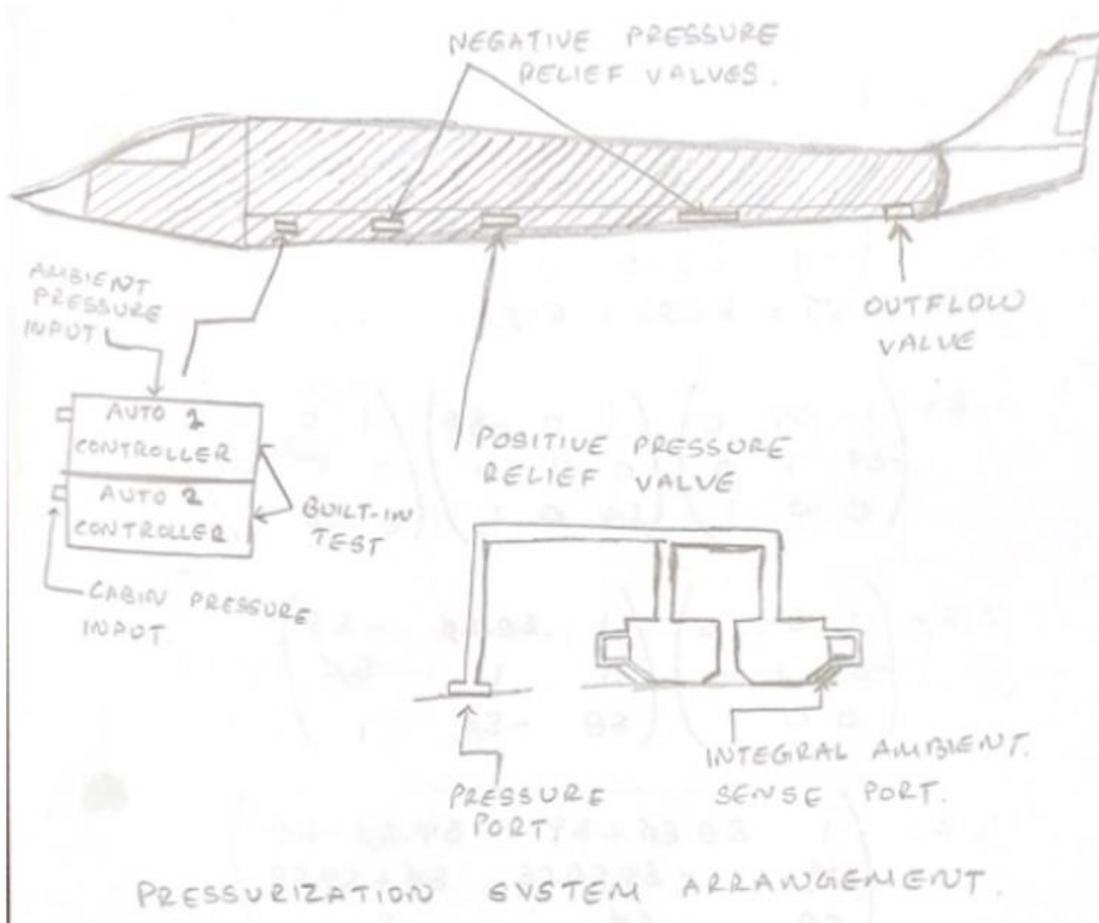
Figure 8: Pressurization System for the TSBJ
