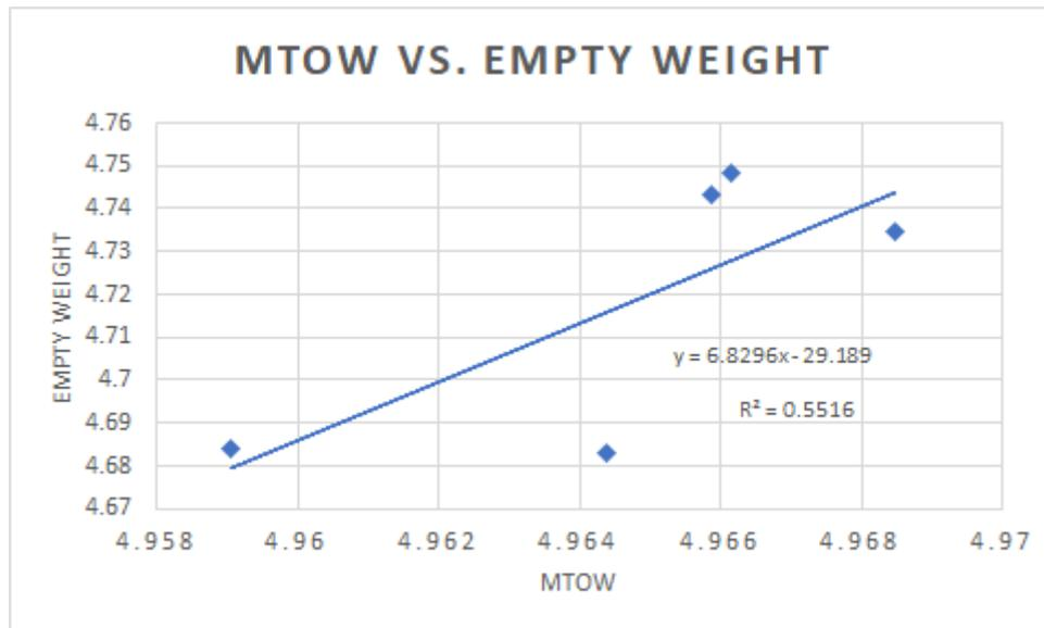
**Figure 2: Graph of the MTOW vs Empty weight**
