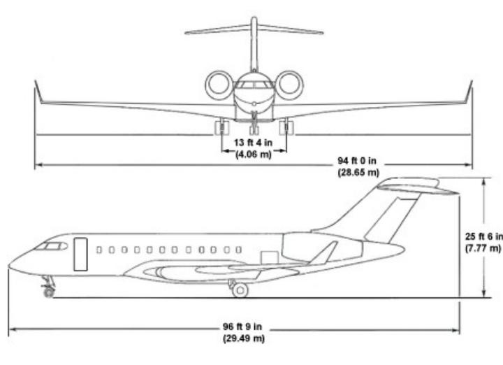
**Figure 2.5: Bombardier Global 5000 Three View Drawing**
