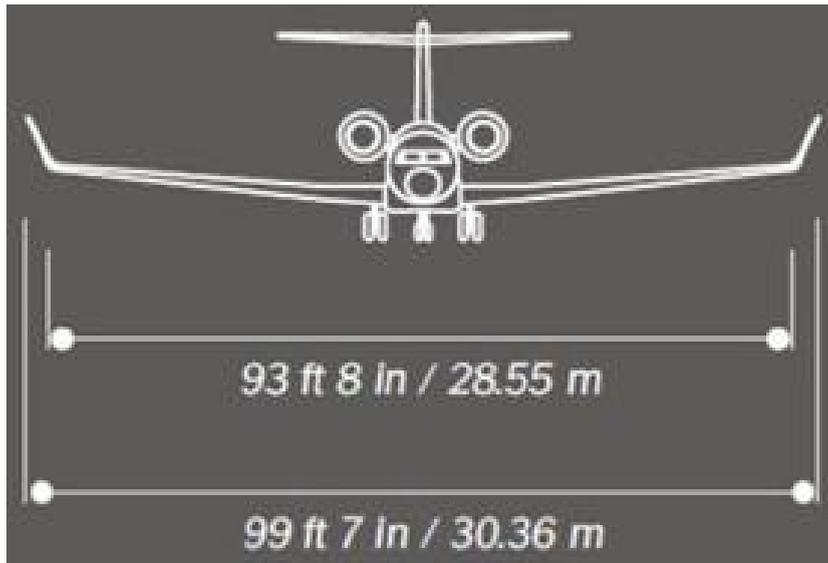
**Figure 1.3: Front view of Gulfstream G650**
