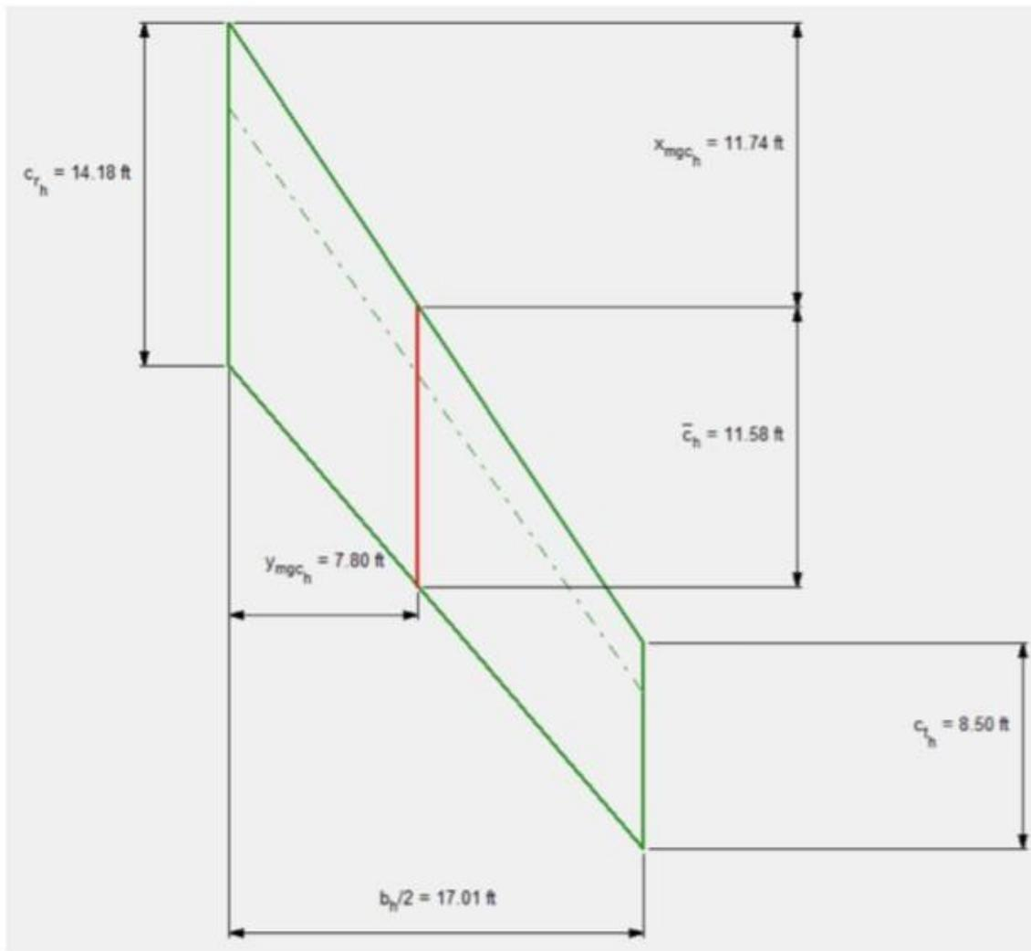
Figure 104: Horizontal Tail Obtained From AAA
