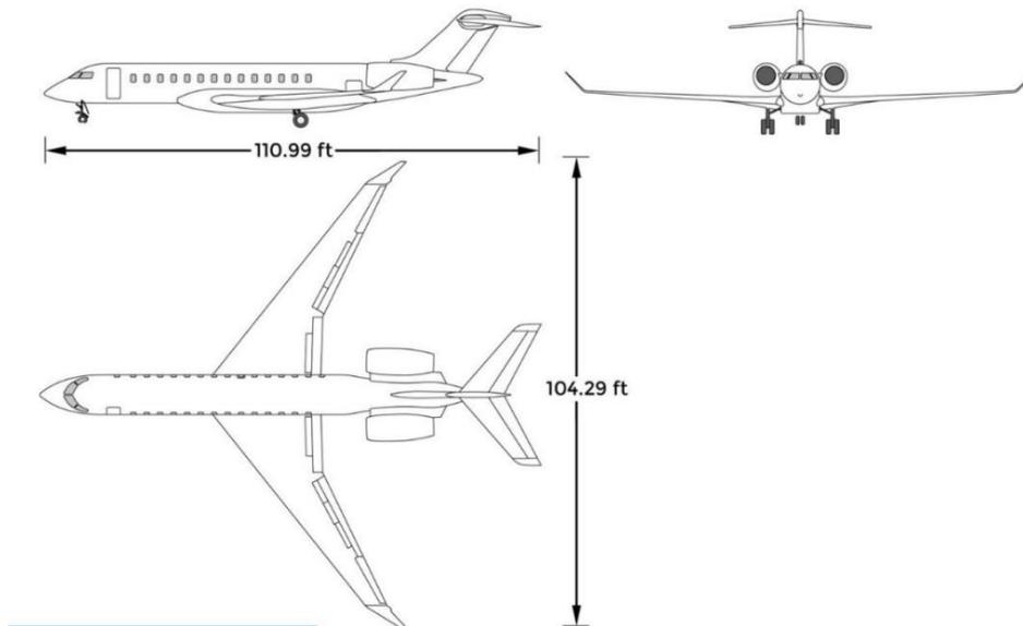
**Figure 2.7: Bombardier Global 7000 Three View Drawing**
