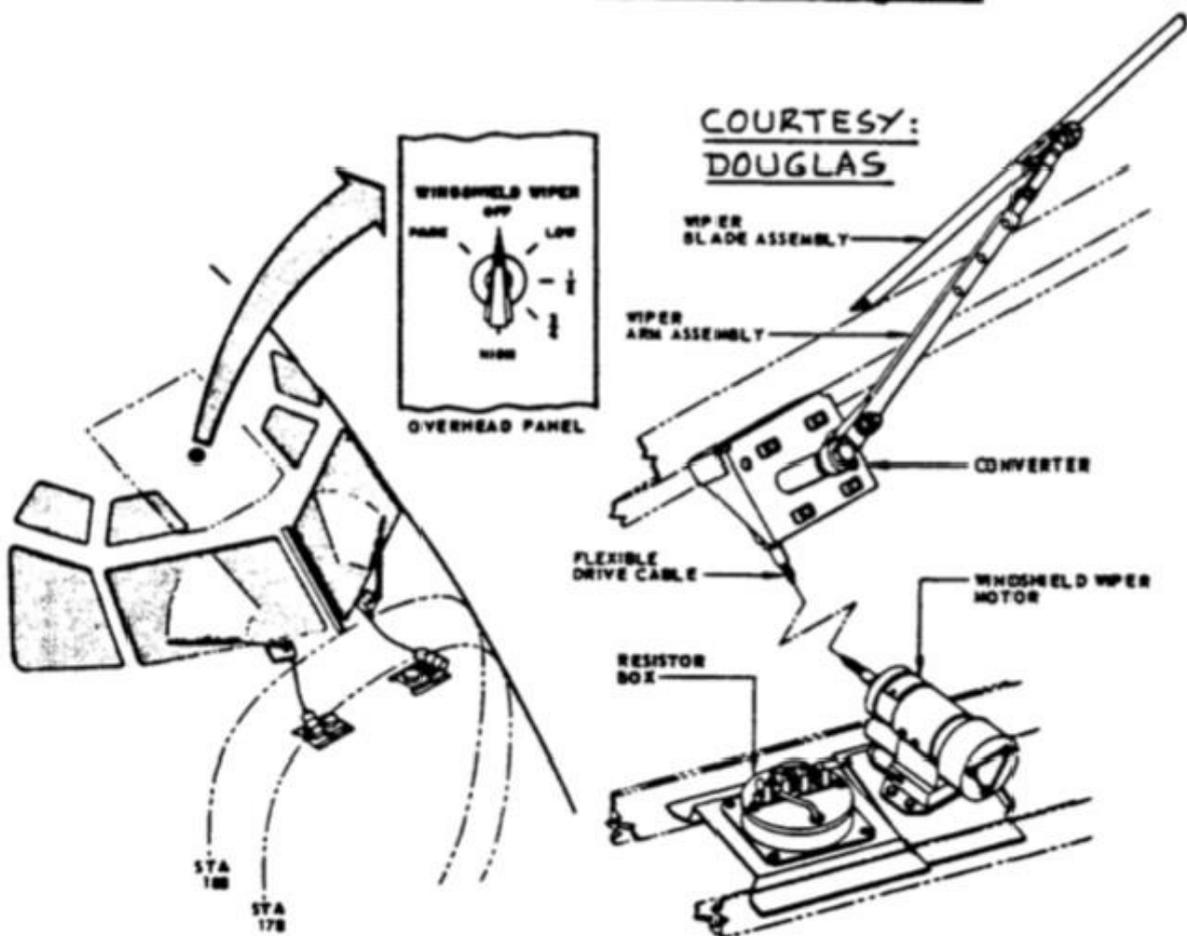
Figure 14: Rain removal system using wipers similar to those in cars.
