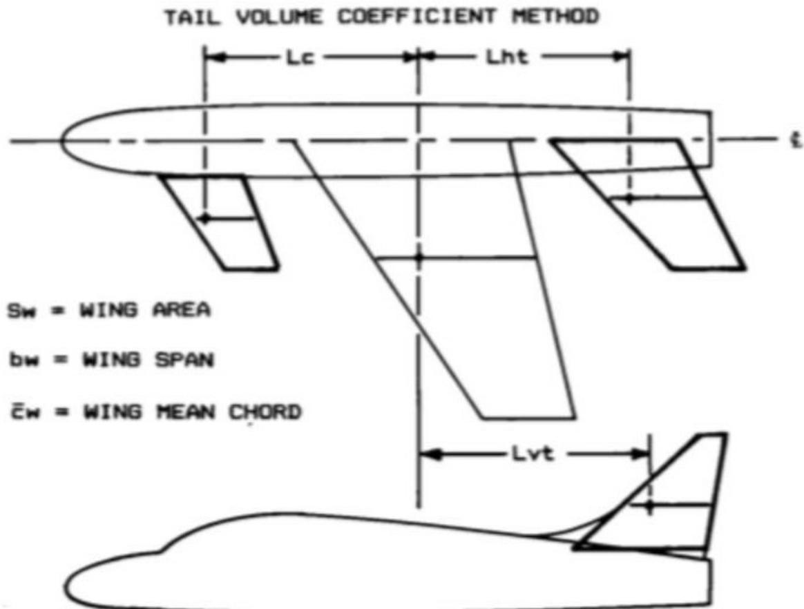
Figure 94: Tail volume coefficient method
