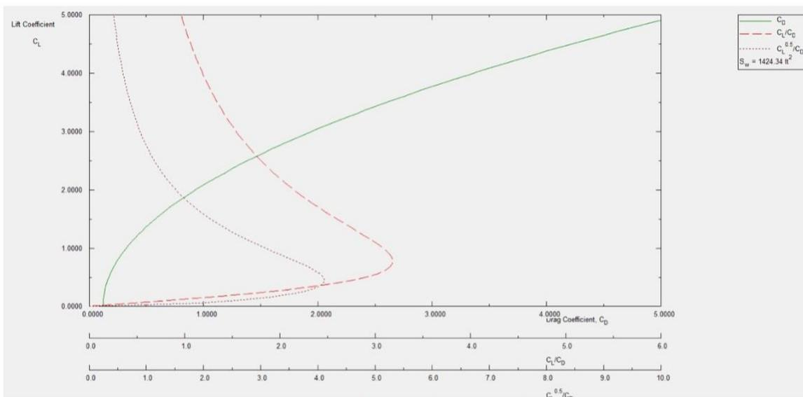
Figure 136: CL v/s CD plots for Landing-Flaps gear down configuration
