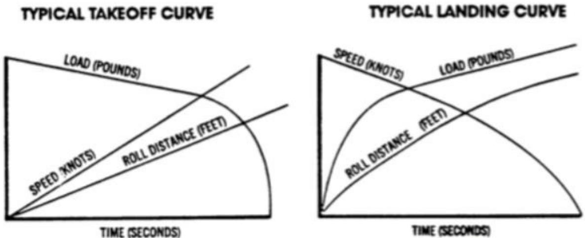
Figure 145: Tire Performance requirements while take-off and landing
