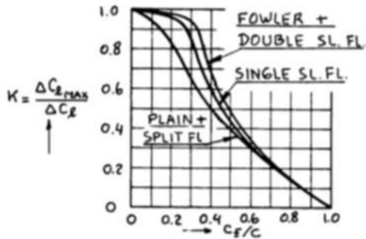
Figure 89: Effect of Flap chord ratio and Flap type on K.
