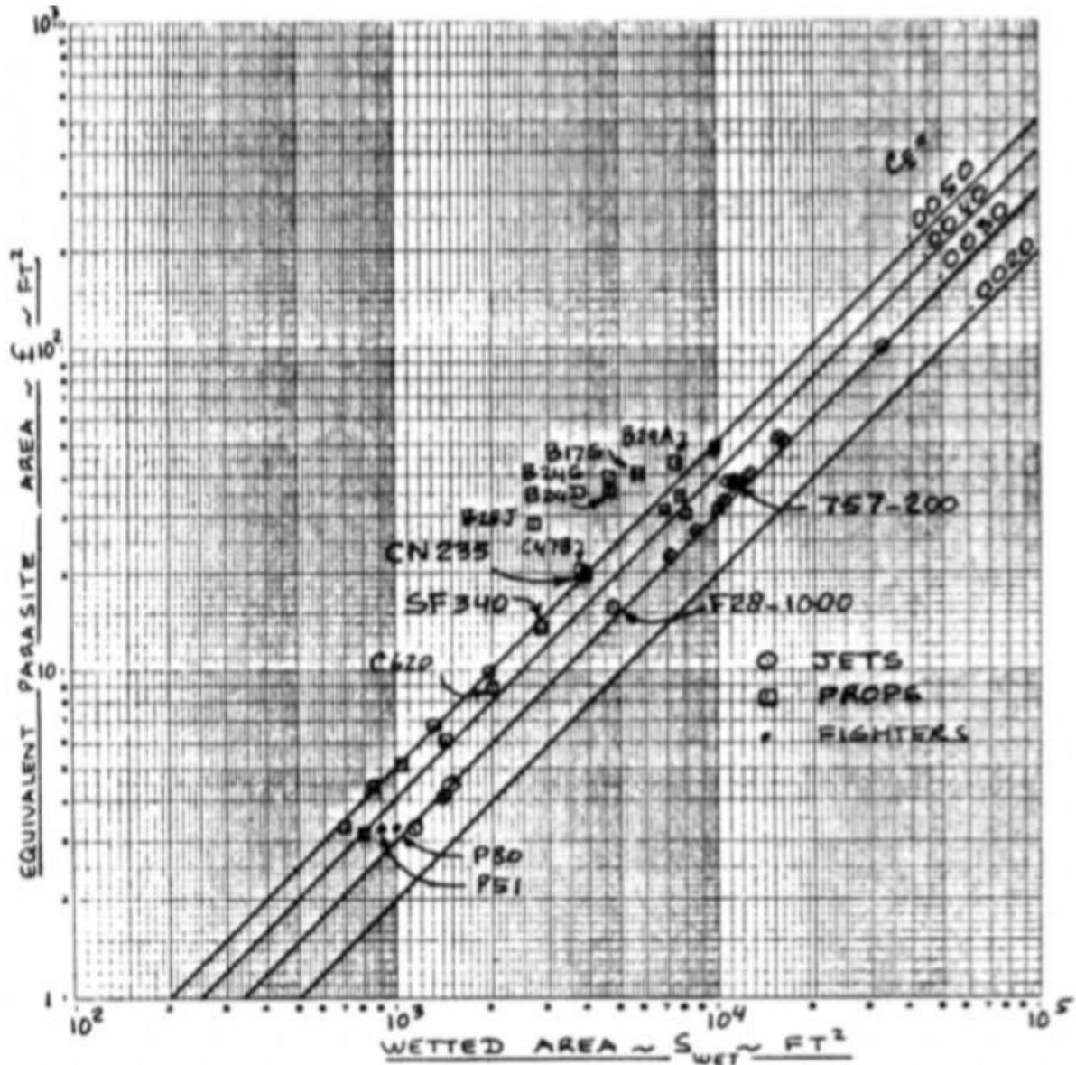
Figure 125: Equivalent Parasite Area v/s Wetted Area
