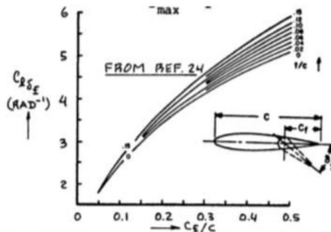
Figure 88: Effect of thickness ratio and chord ratio on  $C_{l_{\delta_f}}$ .
