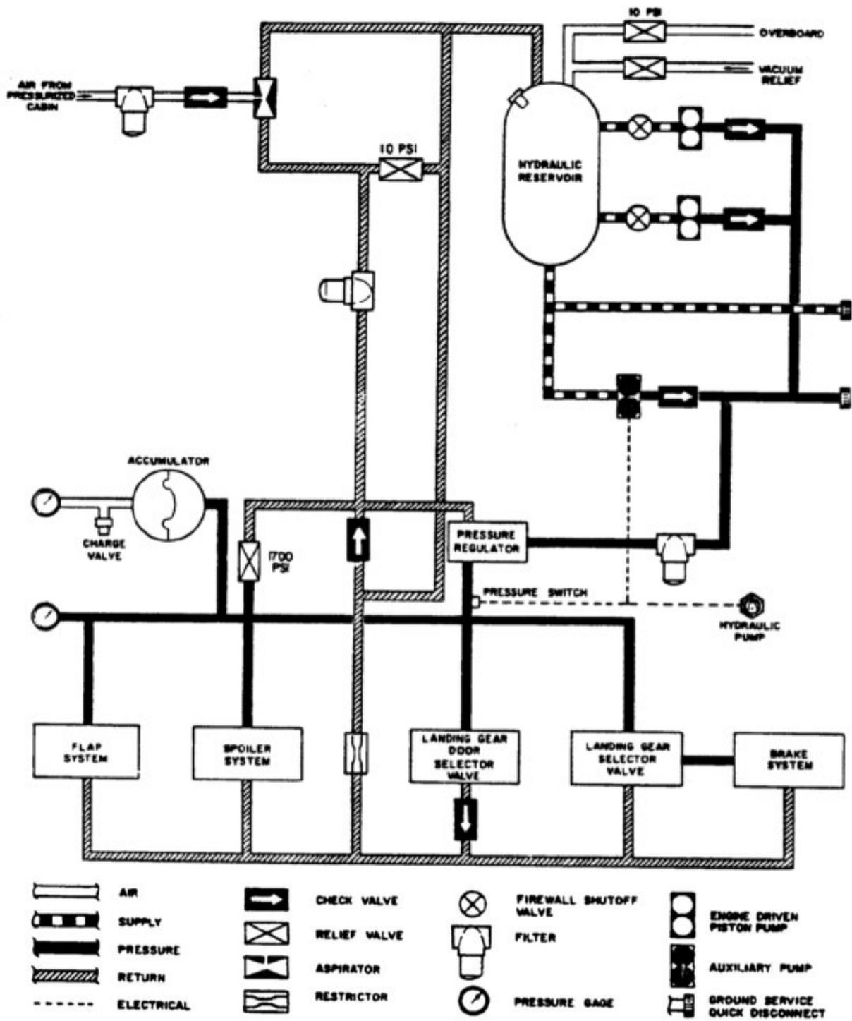
Figure 6: Hydraulic Reservoir of the TSBJ
