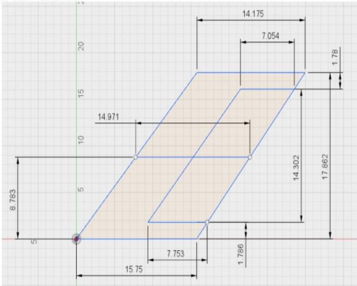
Figure 107: Rudder and vertical stabilizer dimensions (all dimensions in fts)
