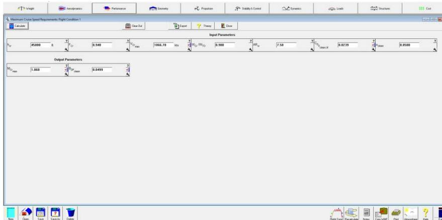
Figure 41: Cruise speed calculations using the AAA program
