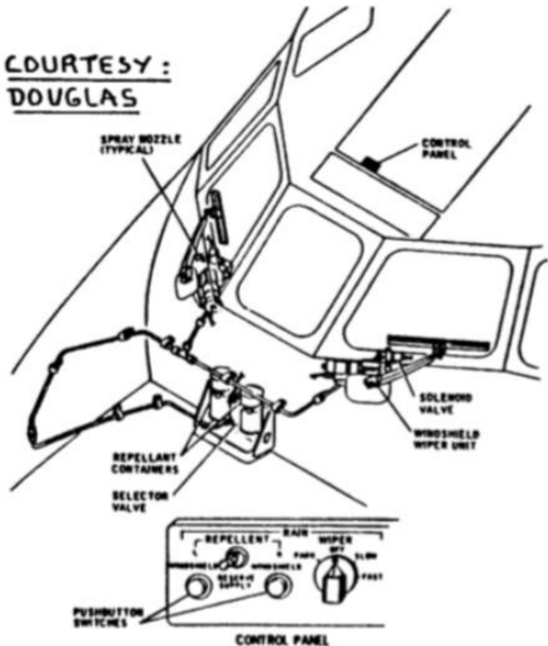
*Figure 15: Rain repellent system added to the wiper paths*
