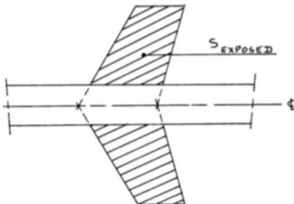
Figure 123: Definition of the Exposed Planform
