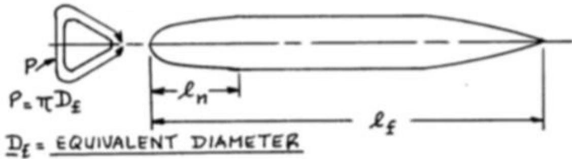
Figure 124: Fuselage Wetted Area Parameters
