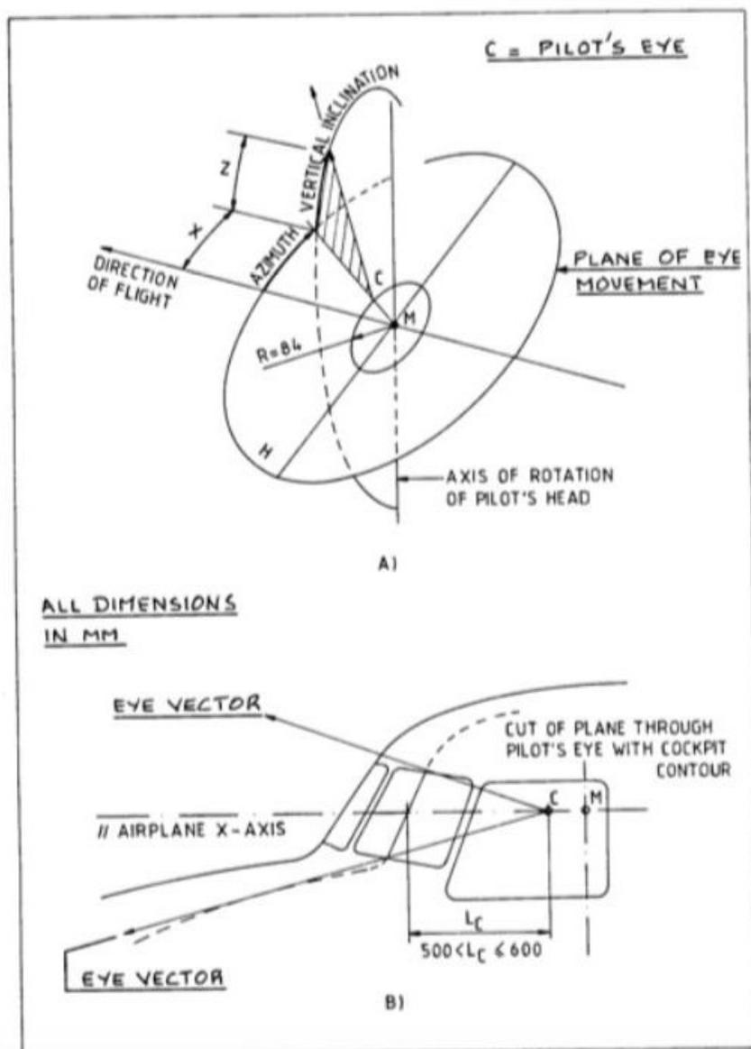
Figure 49: Definition of radial eye vectors
