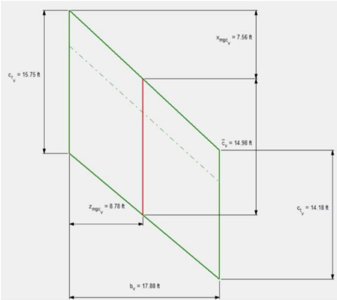
Figure 100: Vertical Tail Obtained From AAA
