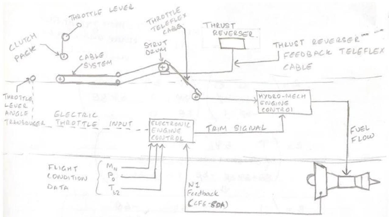
Figure 2: Thrust Control System for the TSBJ
