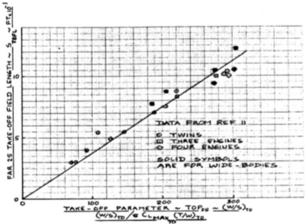
Figure 26: Effect of take-off parameter, TOP 25 on FAR 25 take-off field length
