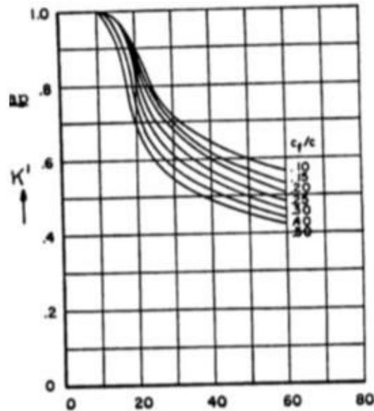
Figure 91: Relation between the flap angle and  $K'$
