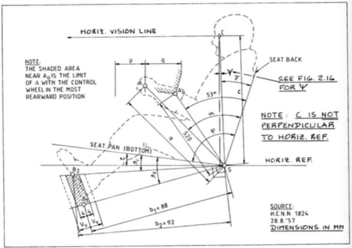
Figure 45: Pilot seat and controls arrangement
