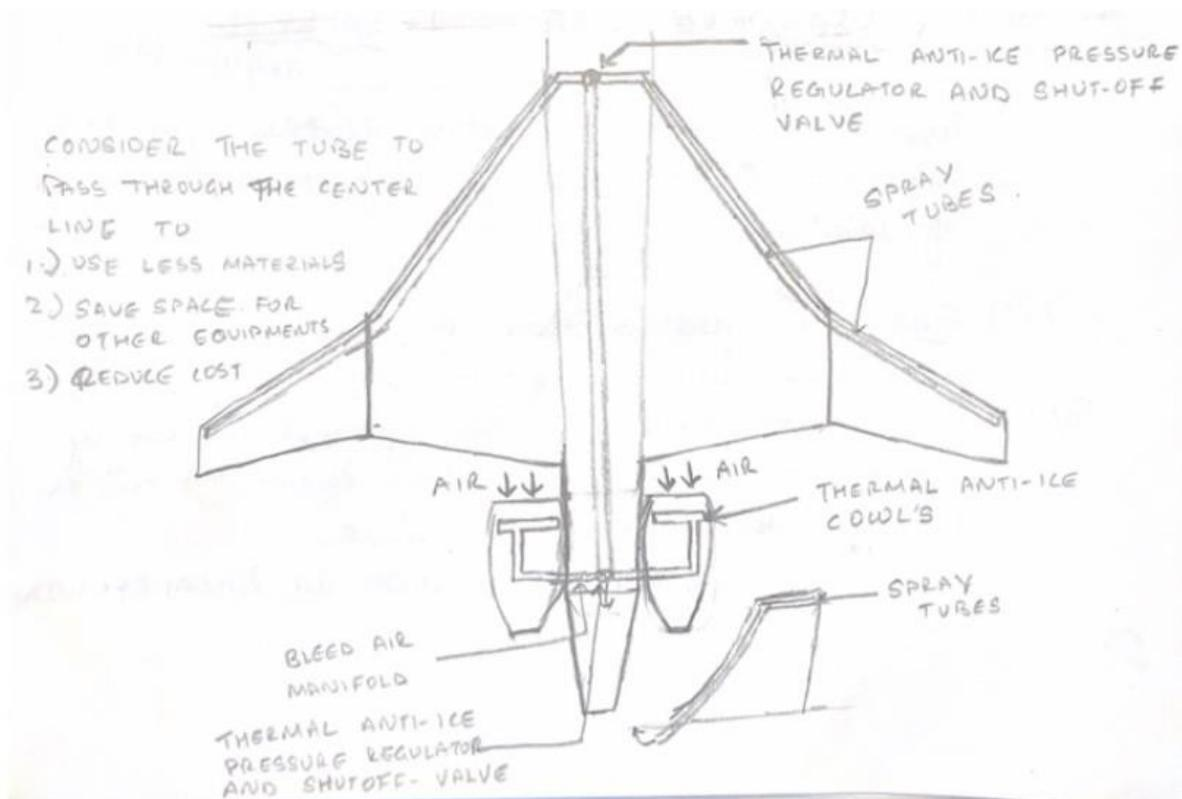
Figure 13: Air Heated Anti-Icing/De-Icing system for the TSBJ
