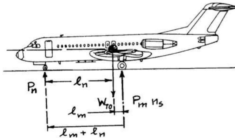
Figure 115: Geometric Wheel location Definition
