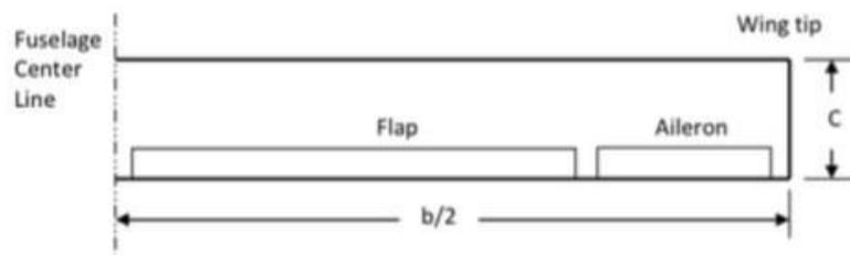
Figure 87: location of high-lift devices on the wing.
