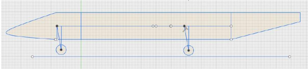
Figure 118: Side View of the TSBJ showing the landing gear Placements
