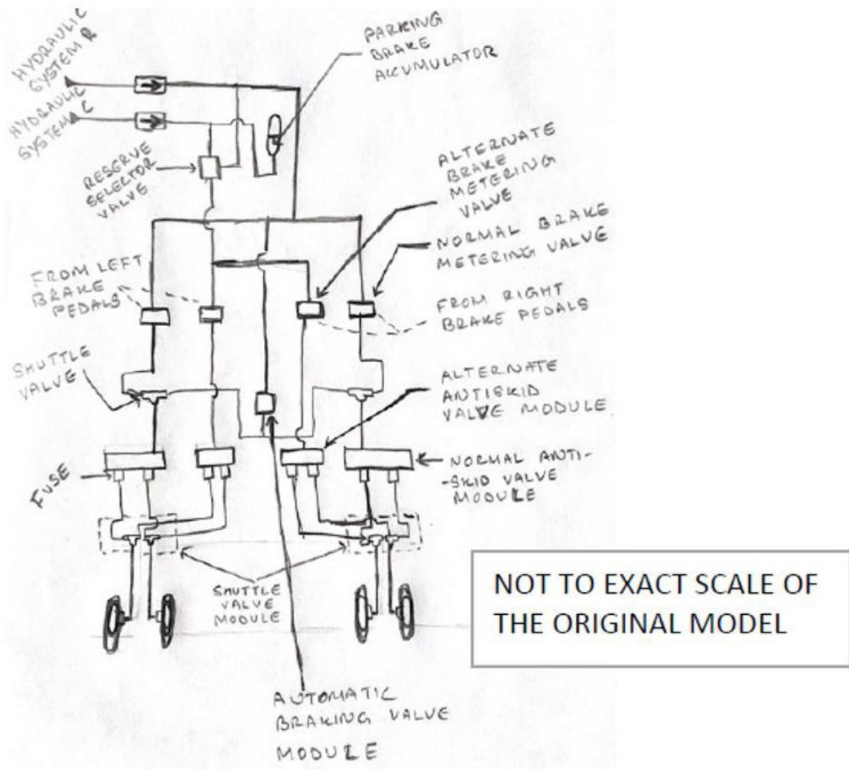
Figure 3: TSBJ Main Landing Gear Control System
