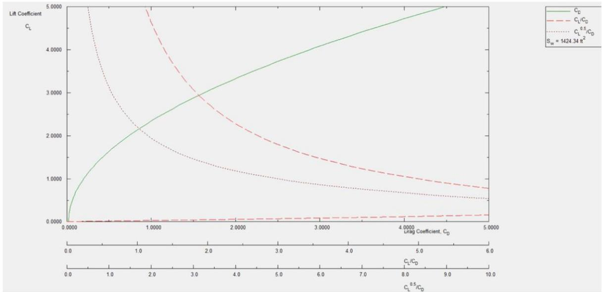
Figure 128: Plot of Clean stage  $C_L$  v/s  $C_D$
