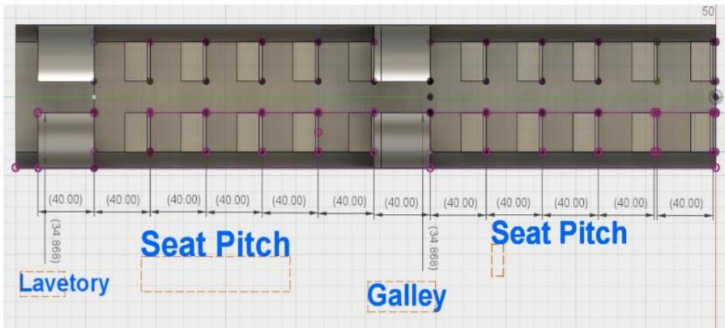
Figure 71: Top view of the interior layout of the fuselage (all units in inches)
